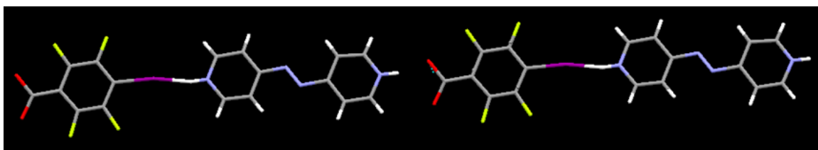
Fig.7 1-D infinite chain in 4,4'-azpy:COOH-I co-crystal formed via O-H...N (py) and C-I...N (py) hydrogen and halogen bond, respectively. For specific information about the crystallography, see the experimental section
