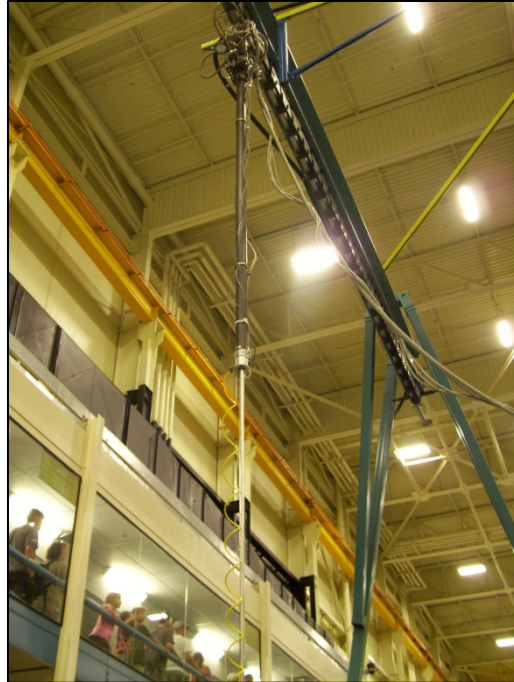
Figure 1-3: The piston on the POGO simulator [1]
