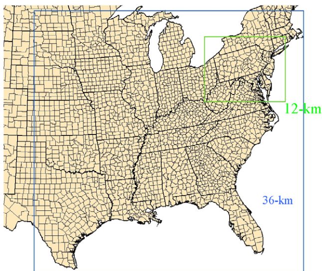
Figure 1. Air quality modeling domain considered for this study; blue box outlines grid modeled at 36 km resolution, green box outlines grid with 12 km resolution.
