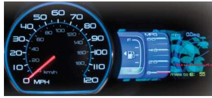
Figure 1.4: The Ford Smartguage EcoGuide increases the efficiency of hybrid power-trains (Ford Motor Company, 2011)
