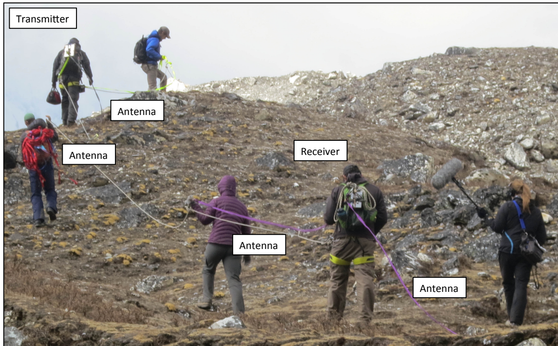
Figure 5. Backpack mounted GPR system deployed in the field at Imja Lake. (Photograph: Alton Byers)
