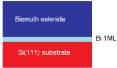
Fig. 2: Side view of the Si/Bi/Bi 2 Se 3 structure.
