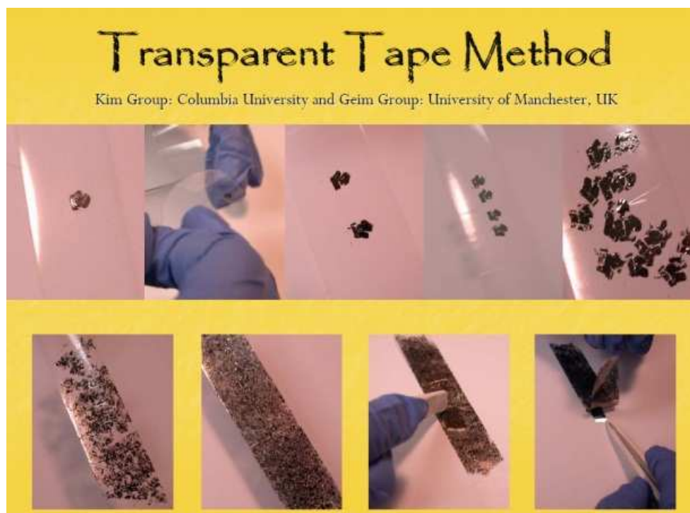
Figure 2.3: Mechanical exfoliation of graphene flakes from a natural graphite chunk onto a \text{SiO}_2 substrate.
