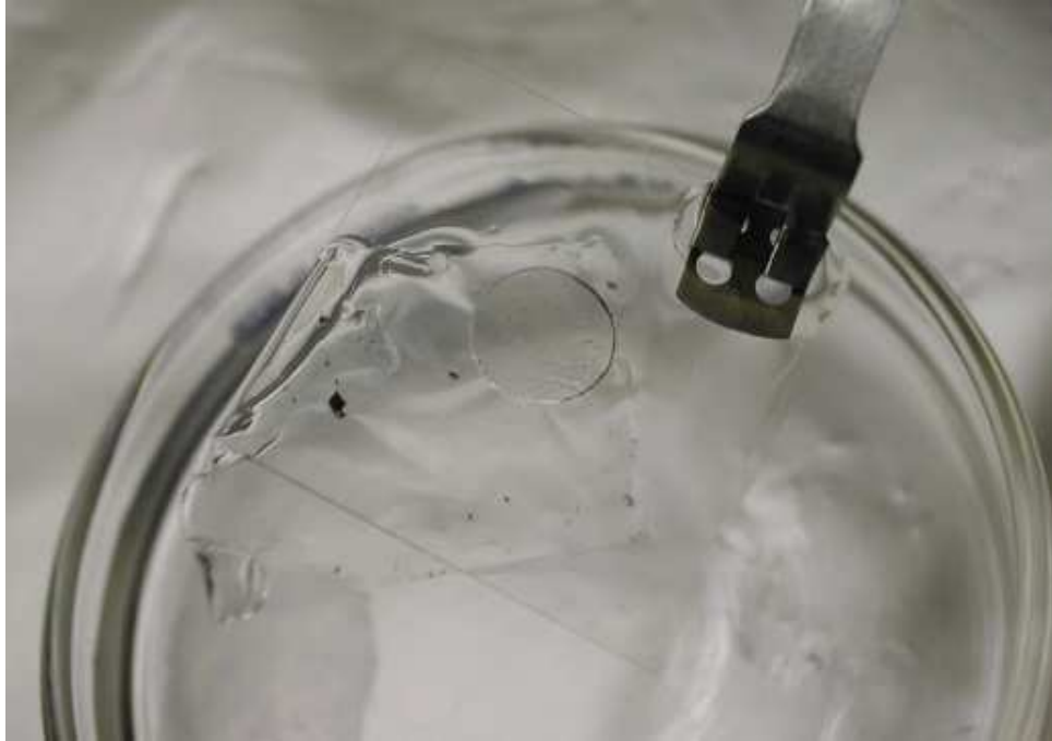
Figure 2.7: PMMA membrane detached from the substrate. Most of the graphene flakes exfoliated on the original substrate are captured in the PMMA film and detached. Large and thick graphene flakes are visible as black dots. A thin cover glass with a hole is used to handle the film to prevent any strain or damage.
