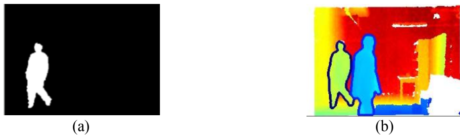
Figure 3.7: (a) Result of our region growth algorithm. (b) The extracted whole body contours are superimposed on the depth map.
