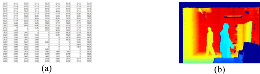
Figure 3.8: (a) a patch of the depth array (b) the depth array showed using color map JET
