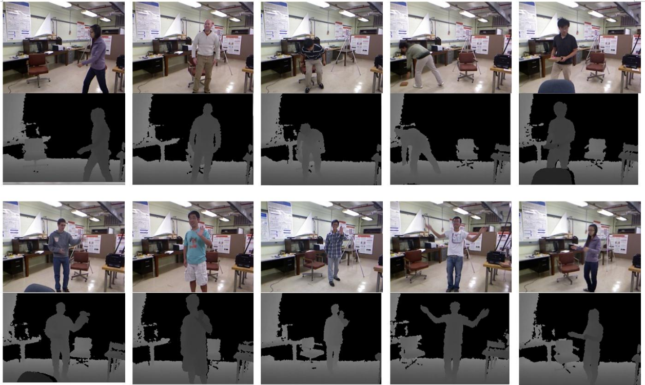
Figure 4.7: Sample images from videos of the 10 activities in our database. Depth and RGB images are shown. Note only depth images are used in the algorithm. Action type from left to right, top to bottom: walk , stand up , sit down , pick up , carry , throw , push , pull , wave hands , clap hands .
