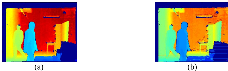
Figure 3.6: (a) Original depth array. Some parts of the body are merged with the ground plane and wall. (b) The input depth array to the region growth algorithm. The ground plane is delineated by the thresholded F filter response. The edges along the feet well separate the persons from the floor.
