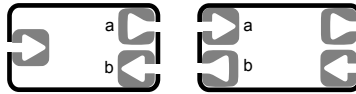
Fig. 3. An example of slightly different process composition than figure 2. The letters indicate the types of the channel-ends that each process takes. It is readily apparent, both that these processes can be composed, and how they should be composed: with a pair of channels.
