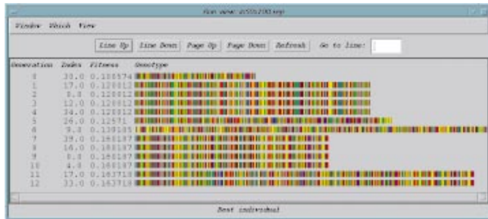
Figure 4.13: An example of a VIS “run window,” illustrating the best individual from each generation using a “zebra” representation.
