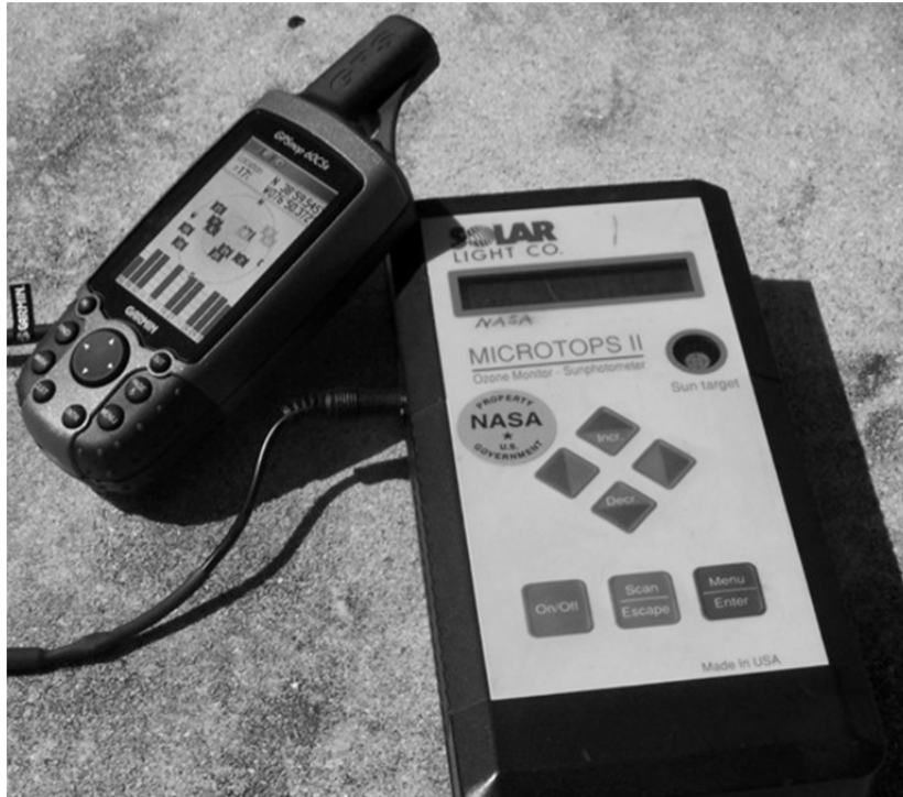
Fig. 5.21 Microtops and GPS unit provided by the Marine Aerosol Network of AERONET at NASA-GSFC.
