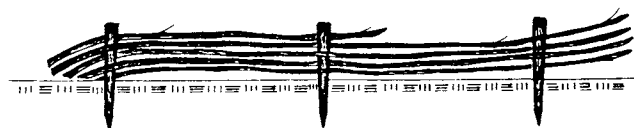
Figure 32. The wattling and staking technique. a. Cross section; b. side view. (Weidelt 1975)
