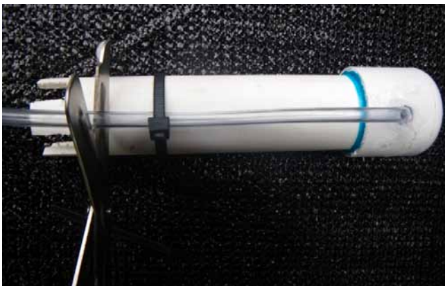
14. Tie the snorkel tube to bell pipe (above) and trim it (below). The bottom end of the snorkel tube should be above the teeth to ensure that air bubbles enter the bell siphon at the right time.
