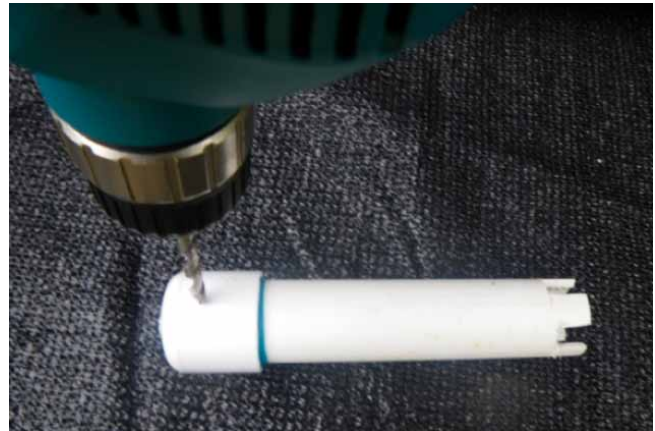
11. Drill a hole in the bell pipe for the snorkel tube.
