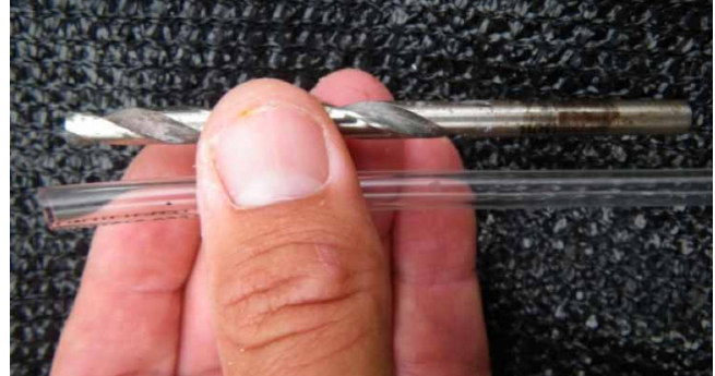
10. Choose the appropriate size (diameter) drill bit or hole-saw for making the snorkel. The hole drilled in the bell pipe should be only slightly larger than the diameter of the tubing itself, to ensure a tight seal.
