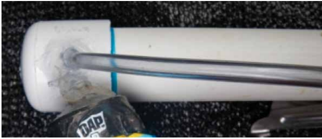
13. Seal the junction of the snorkel tube and bell pipe with 100% silicone. Ensure that the seal is airtight.
