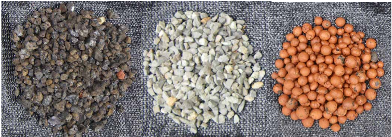
1. Three commonly used solid support media for ebb-and-flow aquaponic systems. Black cinder (left) and pea gravel (center) are produced in Hawai'i; the expanded clay balls (right) typically are imported from Germany.
