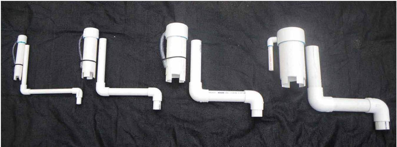
17. Four sizes of bell siphons with accompanying standpipe and drain assembly. From left to right: 1/2-inch standpipe with 1-inch bell pipe; 1-inch standpipe with 2-inch bell pipe; 1 1/2-inch standpipe with 3-inch bell pipe; 2-inch standpipe with 4-inch bell pipe. Note that the top of the standpipe should be even with the bottom rim of the bell pipe when fully assembled in the grow-bed.
