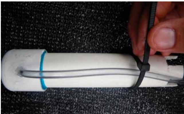
13. Seal the junction of the snorkel tube and bell pipe with 100% silicone. Ensure that the seal is airtight.
