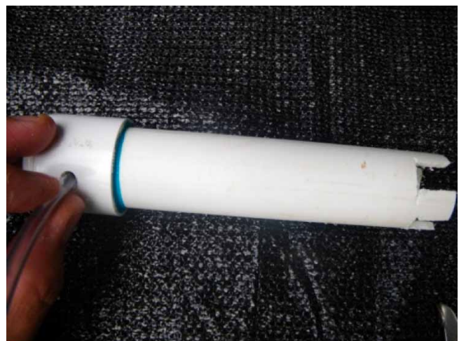
12. Push the snorkel tubing through the bell pipe cap assembly.
