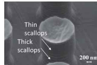
Fig. 13: Micrograph of pillars with slightly stretched scallop marks closer to base of pillar.
