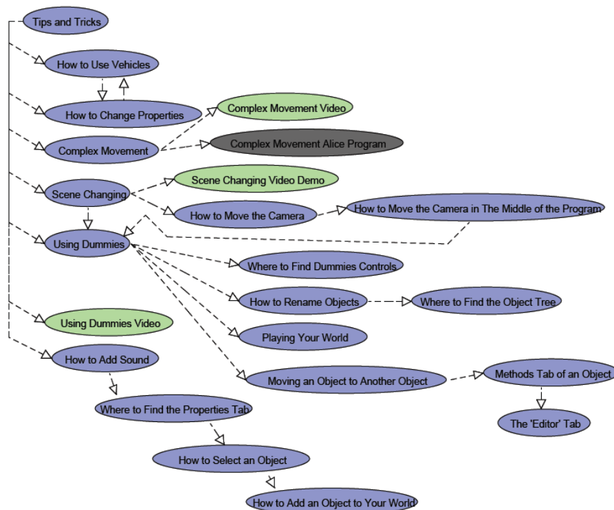
FIGURE 2 AN EXAMPLE OF IETM MODULE BREAKDOWN IN THE TIPS AND TRICKS IETM
