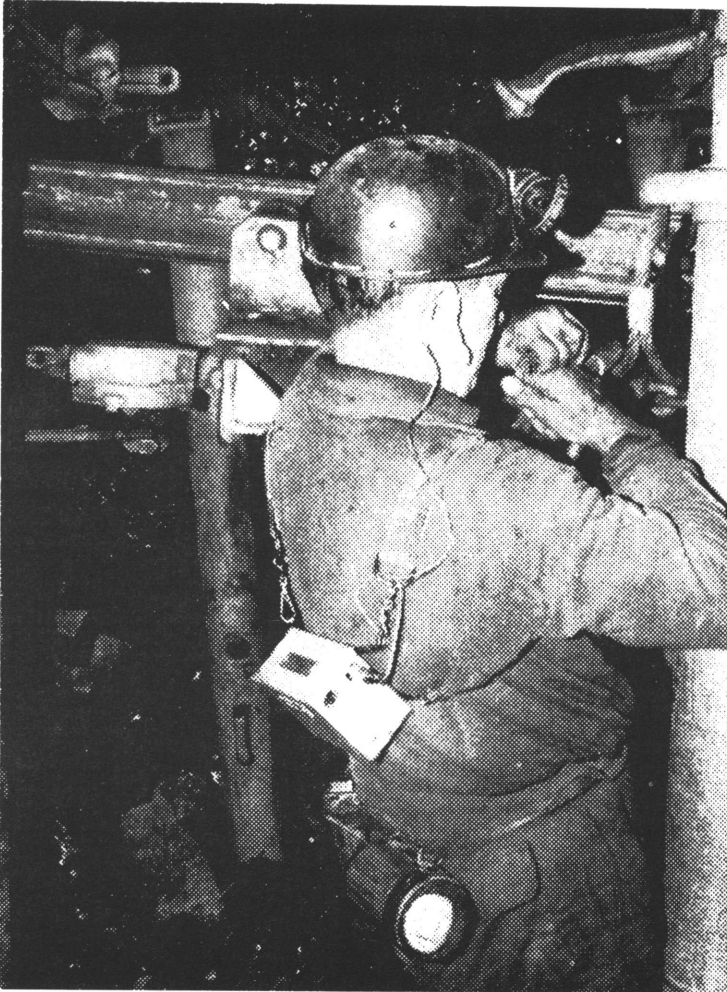
Fig. 5: The firedamp-proof, battery operated pulse counter designed by E. A. MÜLLER, in use.
