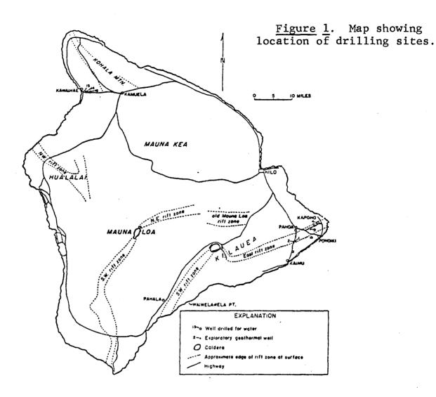
B. Scientific exploratory drilling of 1973. A scientific borehole was drilled to a depth of 4,141 ft. in the region of a marked resistivity anomaly thought to be due to a hydrothermal system. The gradient over the last 100 meters is about 400°C/kilometer and the hole bottom was over 500 ft. below sea level with a temperature of 137°C. (See Table for data.) (Ref. 5).
