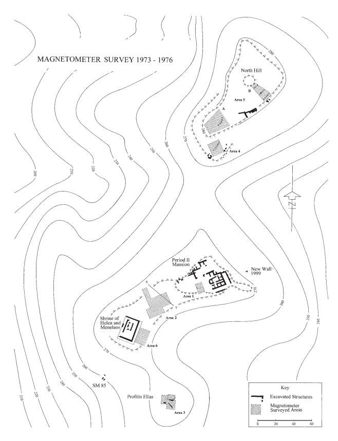
FIG. J.1. Site plan showing Areas 1–6 surveyed with the magnetometer, and for Areas 3-5 the anomalies detected. The anomalies in Areas 4 and 5 (A and B) were observed in individual traverses made within the three areas; they have dotted lines connecting the high intensity locations, shown as small bars approximately 2 m in length. The anomalies in Area  $^{\circ}$  are described in the text.
