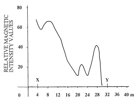
FIG. J.2. Relative magnetic intensity values on the traverse in Area 2. X and Y mark the edges of the plateau.
