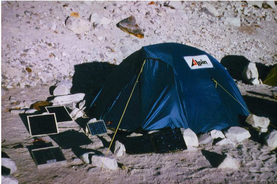
Figure 3. Tent at the base camp at an altitude of 5400 m with solar panels for the laptop devices and satellite telephone for the transfer of the skin resistance data to Germany.
