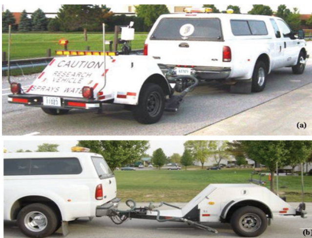
Figure 1.1 ASTM E274 towed friction trailer (a) rear view (b) side view.
