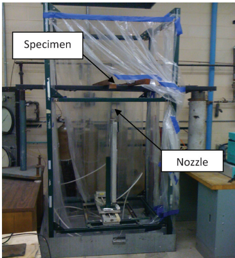
Figure 4.1 Photograph of jet flame test set up.
