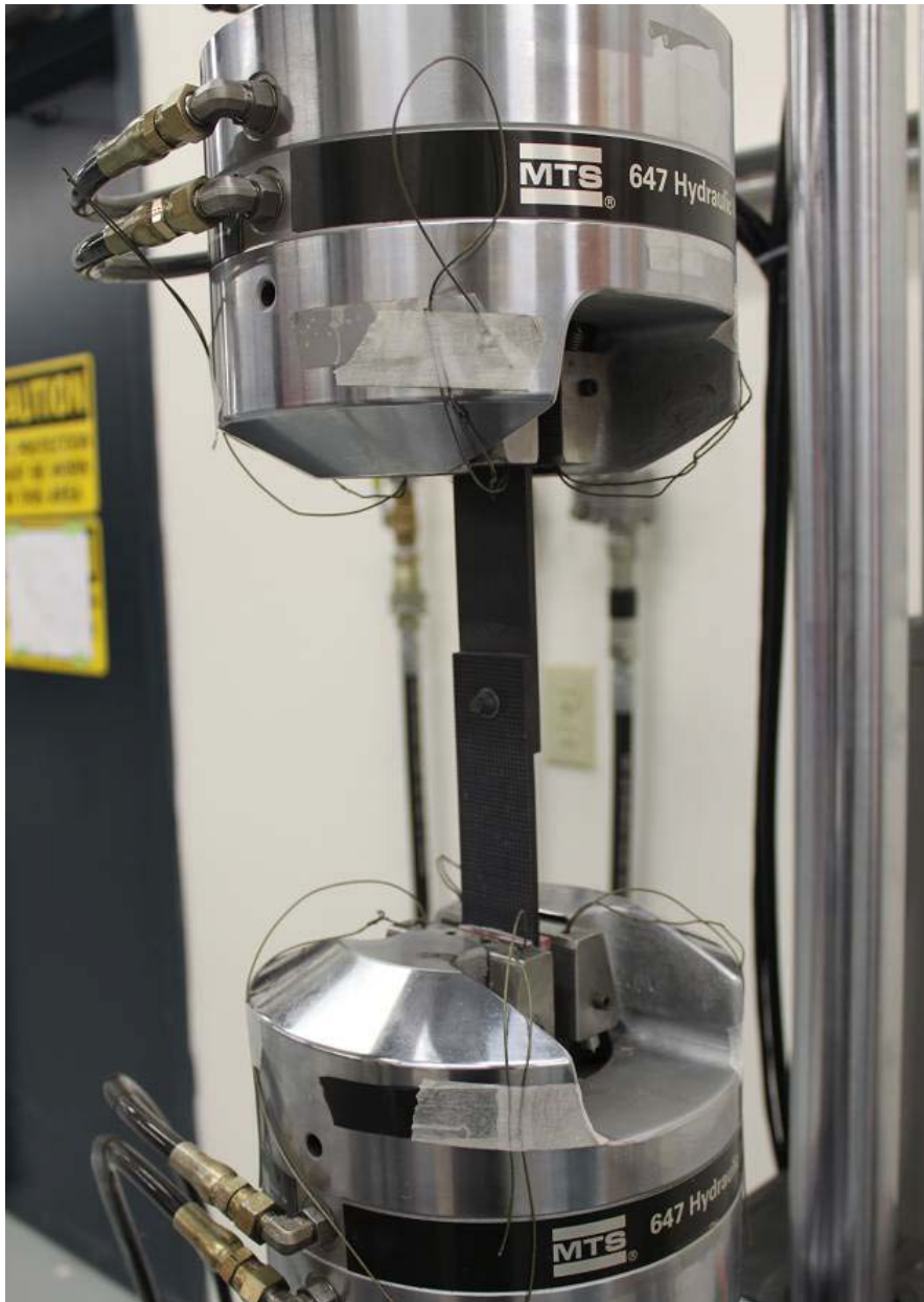
Figure 10. A conventional hybrid joint being tested with the MTS tensile tester.
