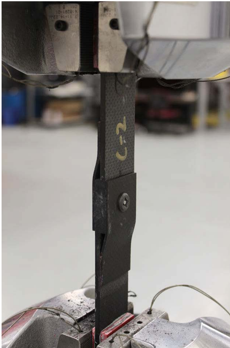
Figure 12. A hybrid joint with curved attachments being tested with the MTS tensile tester.
