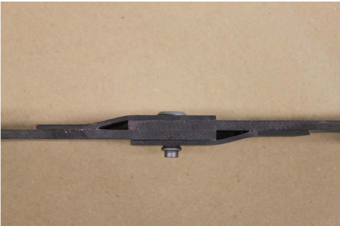
Figure 2. A side view of the hybrid joint with curved attachments.
