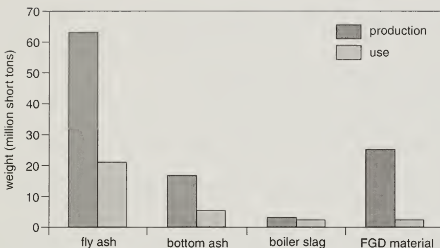
Figure 1 US production and use of CCRs for the year 1998 (plotted using data from ACAA 1999). FGD, flue gas desulfurization.
