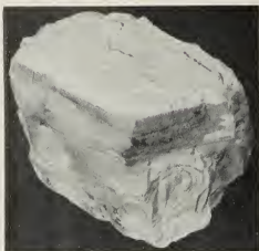
FIG. 10.—Chert from a bedrock outcrop showing the development of a white chalky material on the top of the specimen. Similar material occurs on the bottom but is not visible in the photograph. The white chert in other parts of the specimen is not chalky. About natural size.
