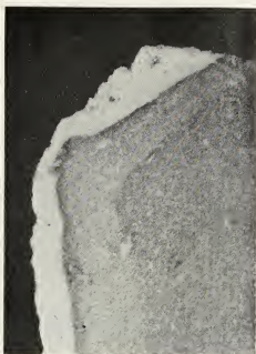
FIG. 9.—Polished section of a "Lafayette" pebble showing white "glaze" over part of exterior, and a light band concentric with the glaze. Reflected light. X 8.
