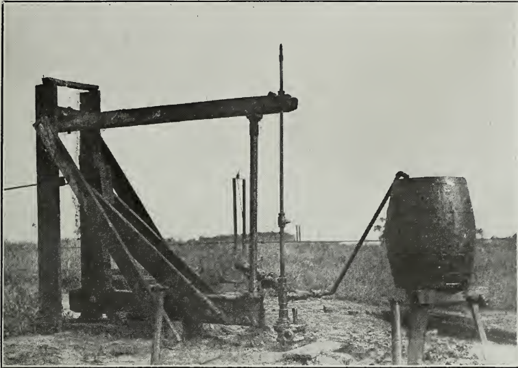
Fig. 24. Photograph of a single-barrel gage setup used early in the work.
