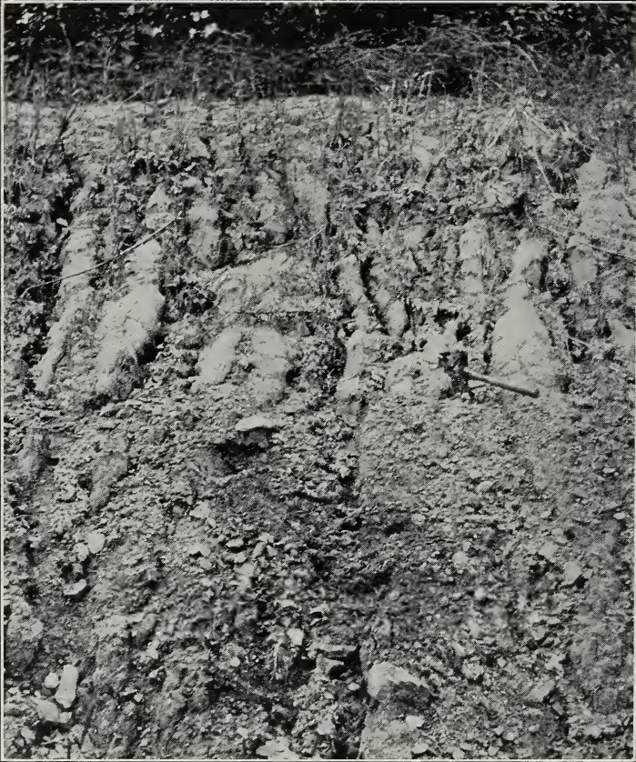
Fig. 37. Peorian loess overlying Illinoian till as exposed in a road-cut near the north margin of sec. 4, T. 14 N., R. 3 W. (Mercer Twp.). A notable pebble concentrate (marked by hammer) occurs on the surface of the till.
