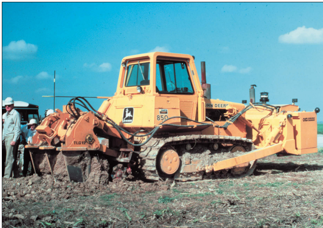
Figure 281 Arch of Illinois, Captain Mine, Perry County. With the new reclamation laws, coal companies required scrapers, bulldozers, and other equipment suitable for handling the soil layers and the more agricultural post-mining phase, as they had to show three years of productivity for prime farm land comparable to pre-mining productivity (Illinois Department of Natural Resources, Office of Mines and Minerals, undated).
