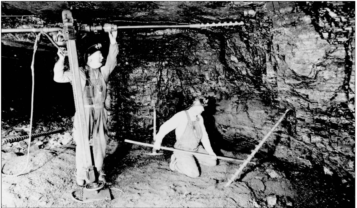
Figure 39 Bell & Zoller Coal Company, No. 1 Mine, near Zeigler, Franklin County. In this scene, miners are operating post-mounted coal drills. In conventional mining (mining that breaks coal by blasting), the face required drilling whether chemical explosives or the breaking agents Cardox or Airdox were used.
