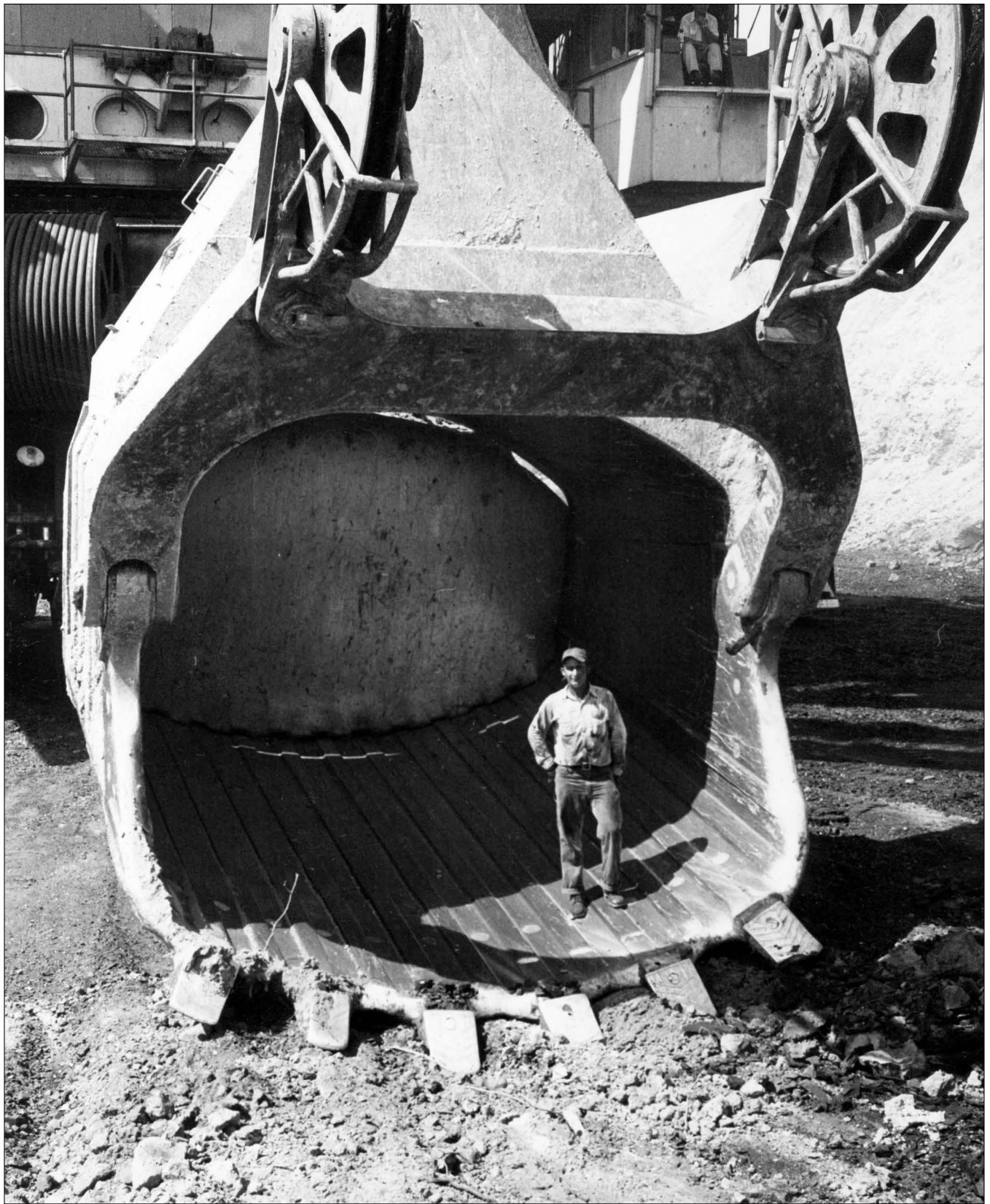
Figure 225 Peabody Coal Company, River King Mine, near Freeburg, St. Clair County. According to a Marion press release, the bucket capacity for the 5760 shovel was 70 cubic yards. The man in the bucket is probably about 6 feet tall.
