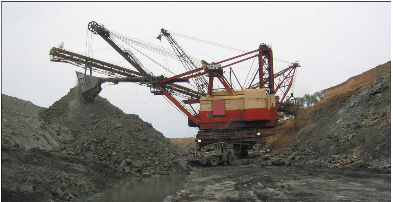
Figure 263 Freeman United Coal Companies, Industry Mine, McDonough County. This Bucyrus-Erie 1050-B stripping shovel had a 45-cubic yard bucket and was purchased in 1960 (Haddock 2001). This shovel was the last operating stripping shovel in Illinois. The mine closed the month after this photograph was taken. Parts of the bucket wheel excavator can be seen behind the shovel.
