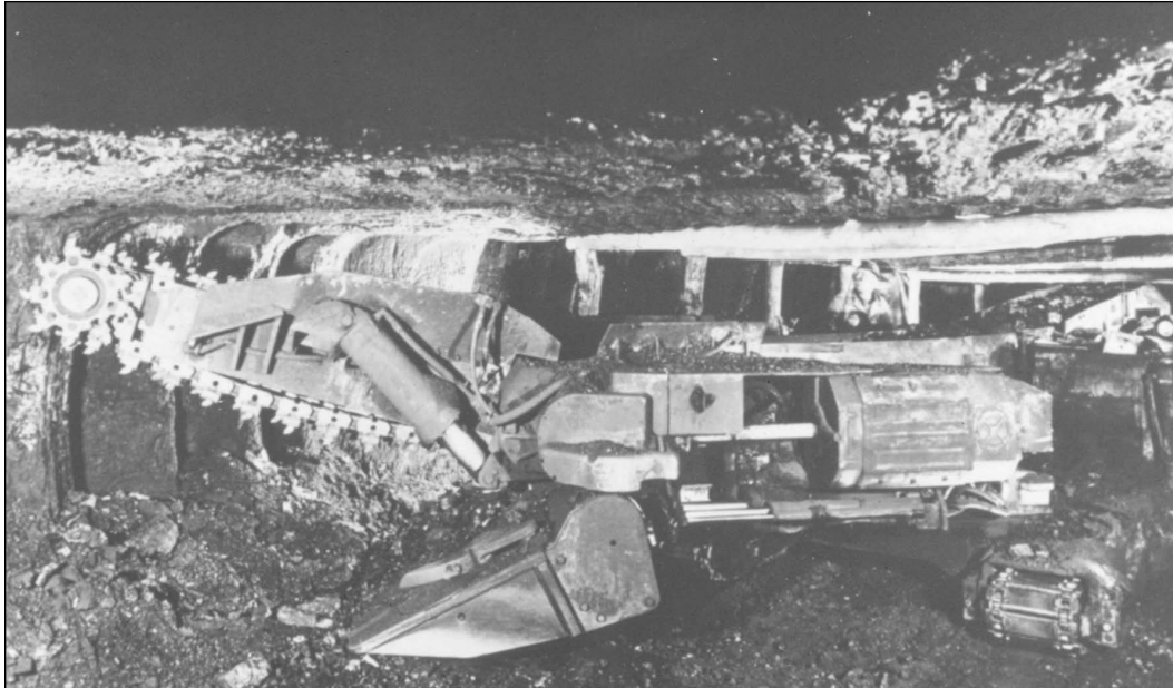
Figure 81 Bell & Zoller Coal Company, No. 3 Mine, near Zeigler, Franklin County. The Joy 1-JCM chain ripper continuous miner shown here shares many parts with a Joy loader, except for the swivel on the crawler section. Modern continuous miners use a drum cutter and lack the swivel feature. This machine could cut 5.5- to 10-foot thick coal and could load at the rate of 5 tons per minute (Ledvina et al. 1992).
