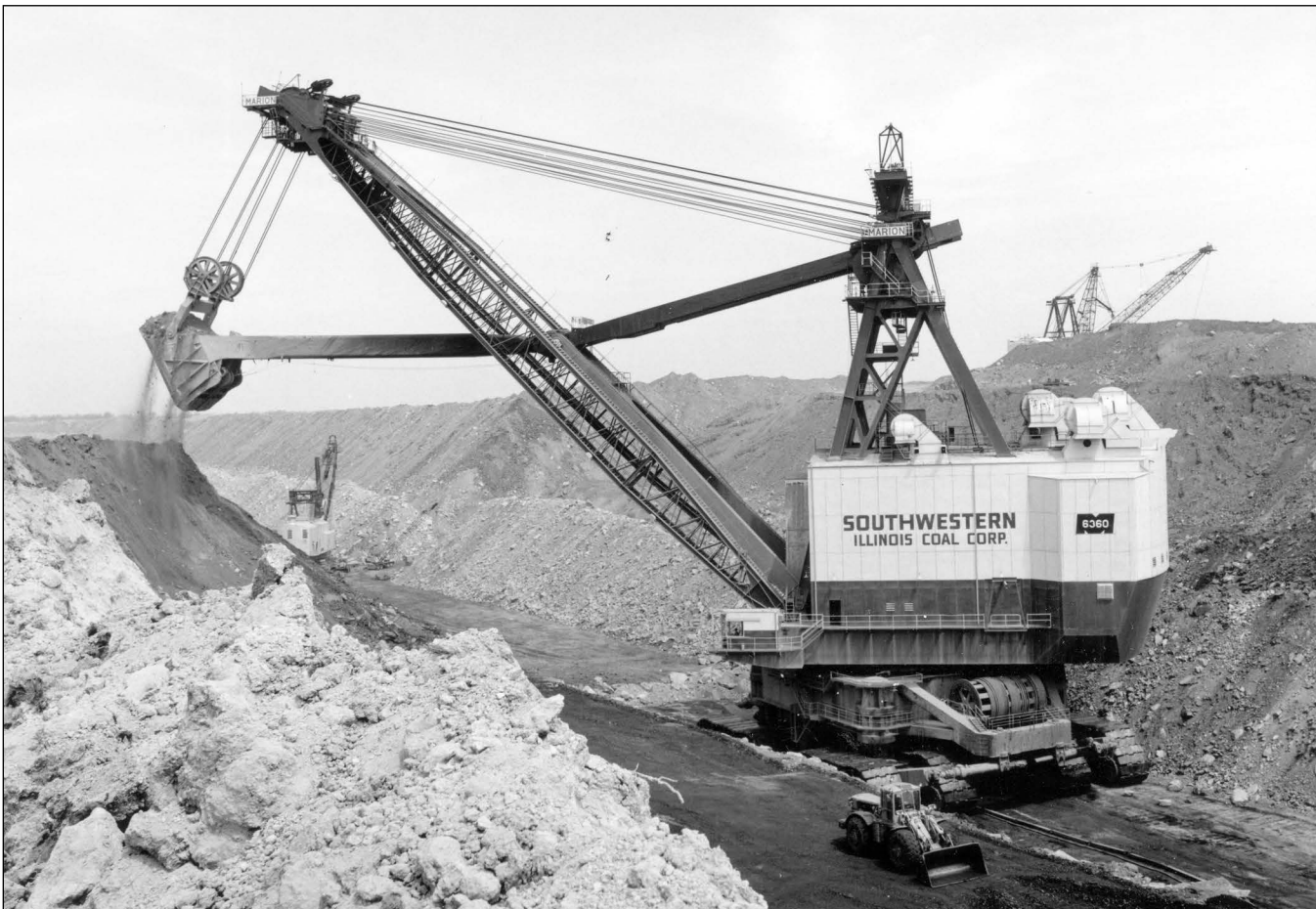
Figure 231 Southwestern Illinois Coal Corporation, Captain Mine, near Willisville, Perry County. “The Captain,” a Marion 6360 stripping shovel, broke all records for size when it was built in 1965. The Captain still holds the record as the heaviest land machine that travels under its own power.
