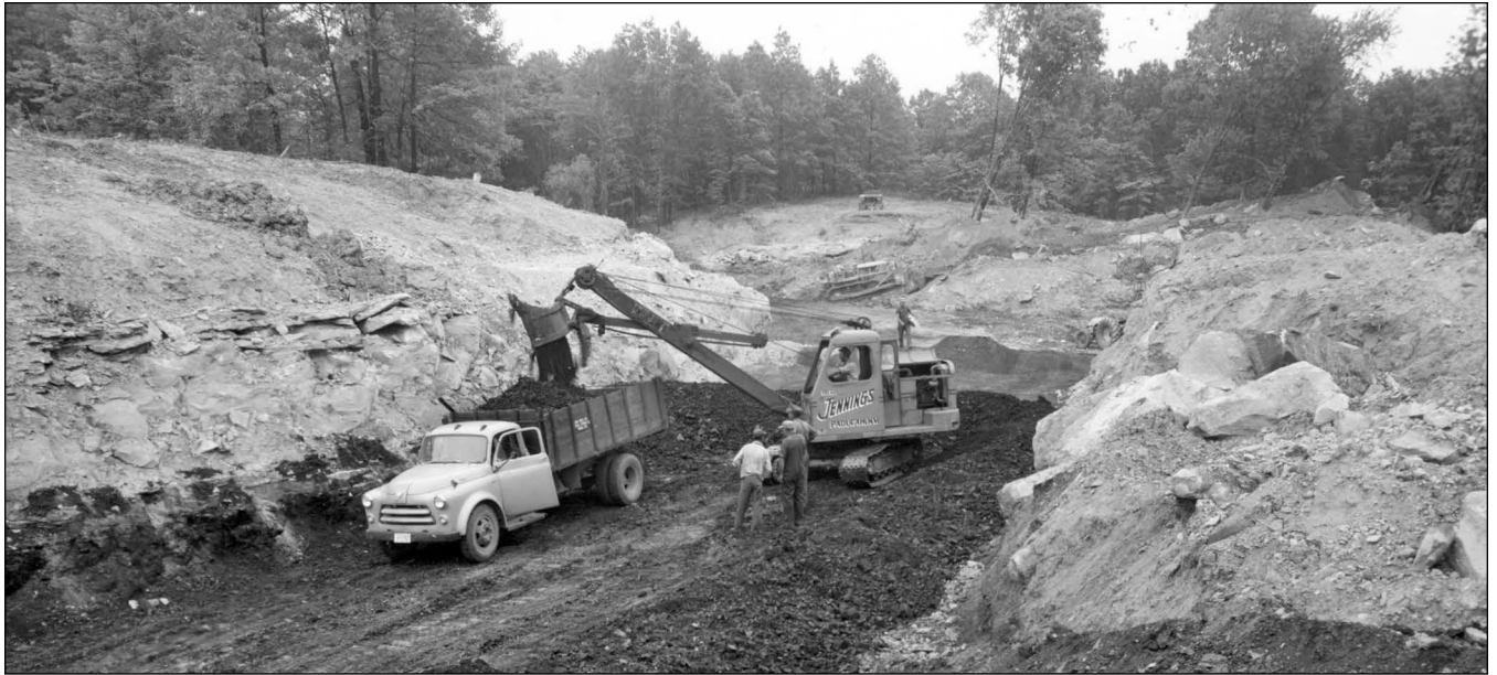
Figure 222 R.C. Jennings Coal Company, Johnson County. Small operations are often called truck-and-shovel operations. They rarely have large stripping equipment, so these operations can move easily from one small parcel of land to another. The sale of coal from a small parcel is not sufficient to purchase a large stripping shovel. Large reserves and large parcels are required for the big equipment.
