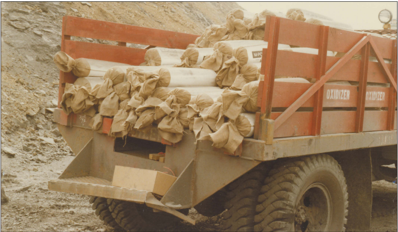
Figure 253 Arch of Illinois, Inc., Captain Mine, near Willisville, Perry County. Tubes of prepackaged ANFO for shooting overburden were brought to the pit, ready to install into horizontal drill holes.
