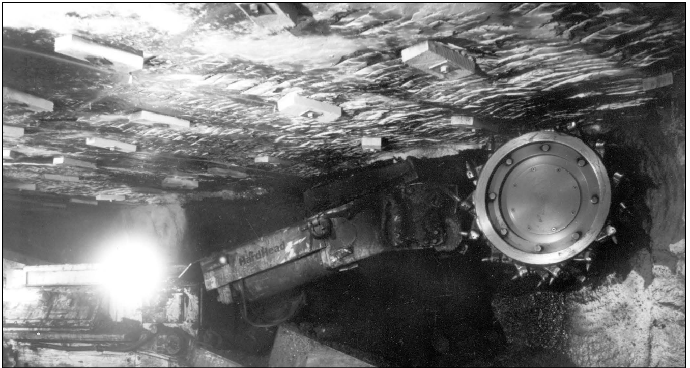
Figure 87 Mine and location unknown. Lee Norse hard head continuous miner. The Joy loading machine was eventually fitted with a series of chains or a drum to cut coal also. The drum design predominated, and the result is the truly modern continuous miner shown here. Drum-type continuous miners may have extendable or fixed width cutting heads or, in some cases, oscillating heads. This is a fixed-width type; hence, the name “hard head” (Ledvina et al. 1992).
