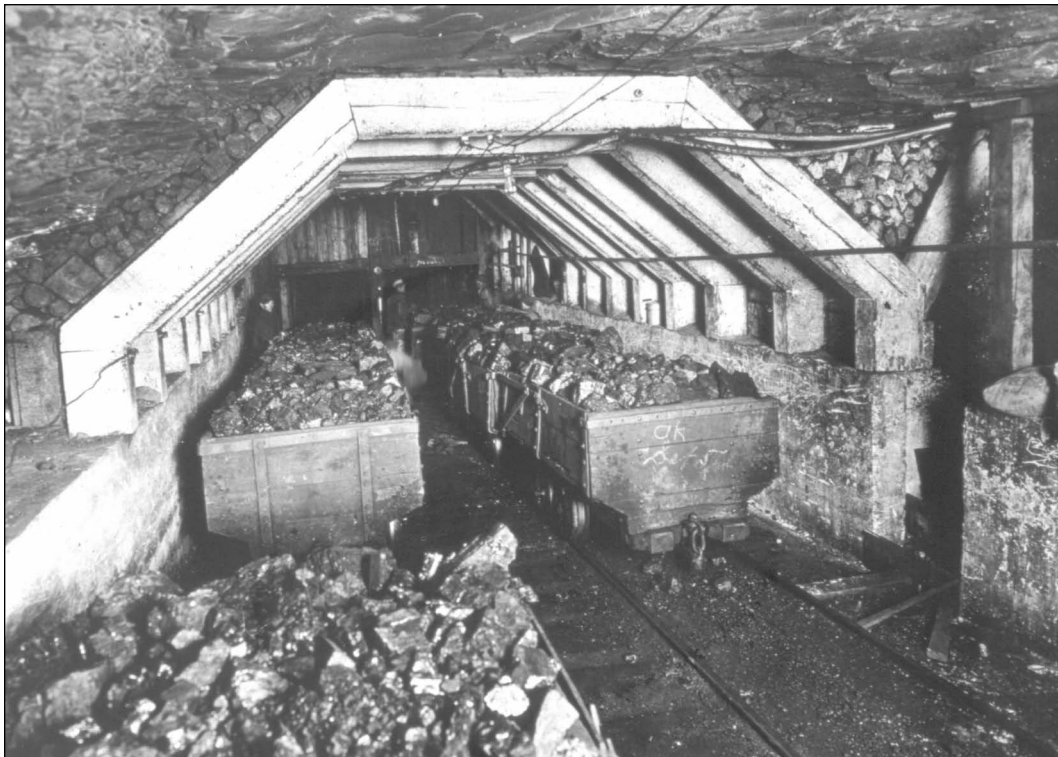
Figure 110 Mine and location unknown. Each car could be maneuvered into the shaft by one man; each car had a man at the front ready to push the empty car off the hoist cage and the loaded car onto the hoist cage. It was critical to keep this area open and free of roof falls. The highly reinforced arch shape is the most stable configuration for roof support.
