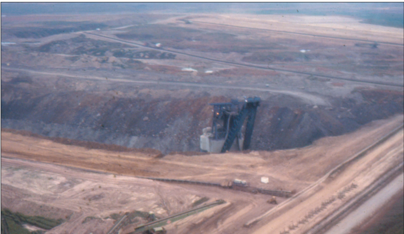
Figure 257 Arch of Illinois, Inc., Captain Mine, near Willisville, Perry County. The large shovel in the center of the photograph is “The Captain.” This photograph shows how reclamation was an integral part of the mining plan. The wheel excavator prepares an area to be mined by removing the subsoil and glacial deposits. These deposits are then transported with the around-pit conveyor to the reclamation area above the shovel (upper right). This efficient technique was developed by the previous owners of the Captain Mine, Southwestern Illinois Coal Company, which practiced reclamation in the 1930s, long before it was required by law.
