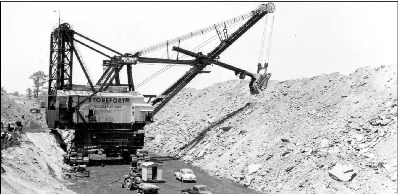
Figure 211 Stonefort Coal Corporation, Will Scarlet Mine, Saline or Williamson County. This Bucyrus-Erie 1050-B was specially designed for the Will Scarlet Mine and two-seam mining. The boom was lengthened from 113 feet to 133 feet, and the bucket size reduced from 36 cubic yards to 26 cubic yards (Dukes 1955). These modifications were needed so that the shovel could make one pass, removing 20 to 50 feet of overburden from the Dekoven Coal to the side and then removing 6 to 17 feet of overburden from the Davis Coal in front of the machine.
