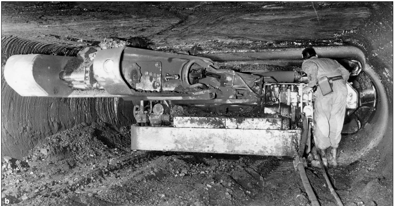
Figure 84 Mine and location unknown. Two views of a boring-type continuous miner. As shown, the miner cuts a curved side wall entry, which provides stability to the roof. These machines had some height adjustment capabilities. This machine had four cutting heads, and each head made an inner circle on the central axis; two outer cutting arms had easily replaceable tapered shank cutter bits. In thicker coal, an extension was added so that three cutting arms were attached outside the inner revolving axis. The distance between the rotary cutting arms could also be telescoped in discrete increments to adjust the machine to any variation in seam height. The top and bottom cutter bars could be moved independently. The miner weighed between 40 and 50 tons and had a capacity of 8 tons per minute. The cutting element could be tilted vertically or sideways or raised or lowered to compensate for seam irregularities (Goodman Manufacturing Company undated). Photograph (b) shows the end of the tail conveyor where coal would come out during mining.
