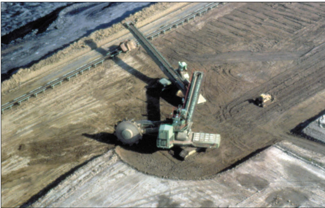
Figure 256 Arch of Illinois, Inc., Captain Mine, near Willisville, Perry County. The O & K wheel excavator moves forward and takes a semicircular “bite” out of the subsoil or glacial drift. The material is then transferred to the Weserhütte conveyor to be evenly deposited onto the around-pit conveyor belt system.
