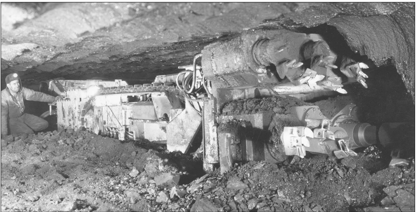
Figure 86 Mine and location unknown. A Jeffrey Manufacturing Company boring-type continuous miner. Coal is shunted back by the operator on a conveyor for transport to the main haulage.
