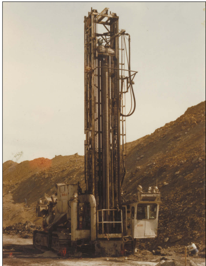
Figure 250 Arch of Illinois, Inc., Captain Mine, Perry County. This rig is drilling holes to shoot the overburden to the Springfield Coal after the Herrin Coal has been mined.
