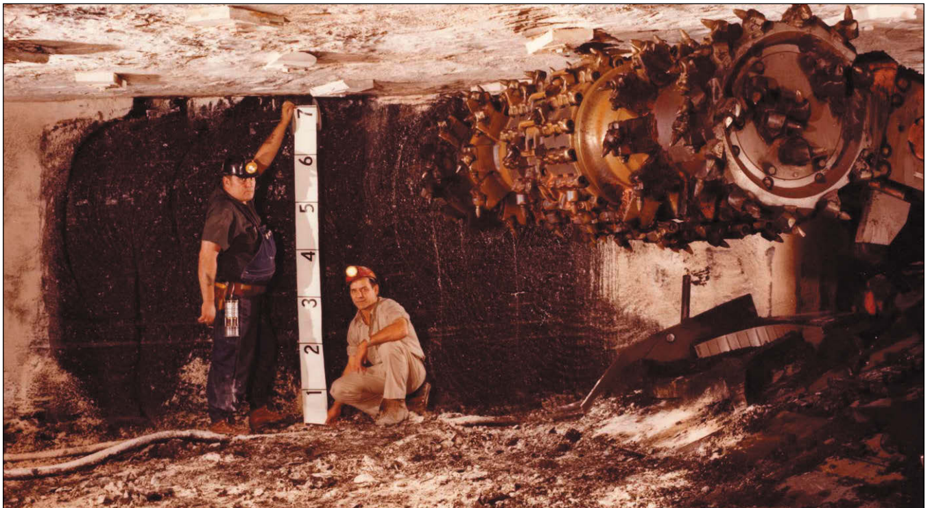
Figure 88 Peabody Coal Company, Marissa Mine, Washington County. This milling-type continuous miner could raise and lower the cutting head while mining the coal and so could mine varying seam heights and coal where the thickness varied.
