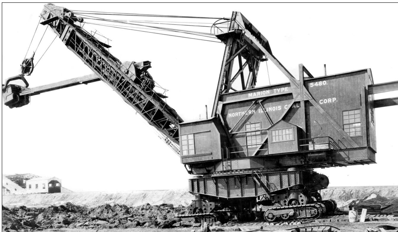
Figure 196 Northern Illinois Coal Corporation, Northern Mine, Will County. The Marion 5480E electric shovel was crawler-mounted and had a 12-cubic yard bucket (Hollingsworth 1963) and weighed 975 tons (Historical Construction Equipment Association 2002). This machine also featured a three-part hoist, inside dipper stick, and rack and pinion crowd. At about this time, Bucyrus constructed Model 750-B, which had twin hoist ropes on the dipper. This model helped eliminate an old shovel problem, when one side of a dipper caught on a rock or hard spot and twisted the front end, cracking the dipper stick or warping the boom (Hollingsworth 1963). The rails extending from the rear portion of the housing are for an internal crane that aided maintenance and repairs. Doors in the back could be opened to bring in equipment (Historical Construction Equipment Association 2002).
