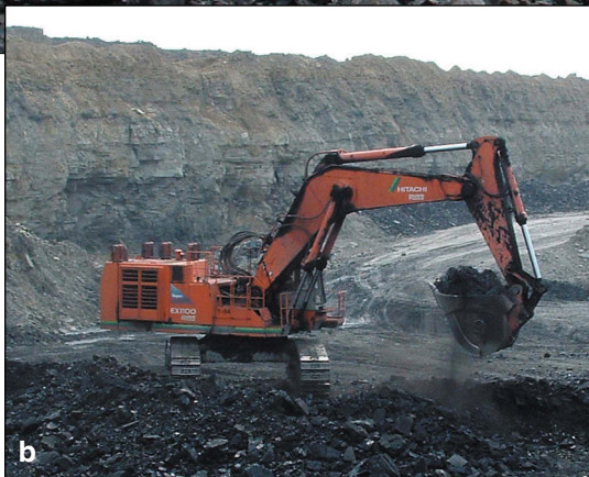
Figure 267 Vigo Coal Company, Wabash County. (a) This caterpillar wheel loader is one of three types used at this mine. (b, c) The Rudd-Hitachi EX1100 loader has a versatile bucket that swings 180 degrees.
