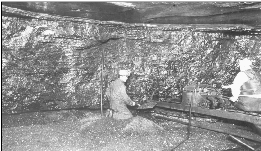
Figure 29 Mine and location unknown. This undercutter uses a type of gathering chain to rip the material from under the coal. The helper shovels the fine coal shavings away from the face. This machine is similar to the early Jeffrey Manufacturing Company undercutters (Morrow 1962). Note the completed cut to the left of the helper.
