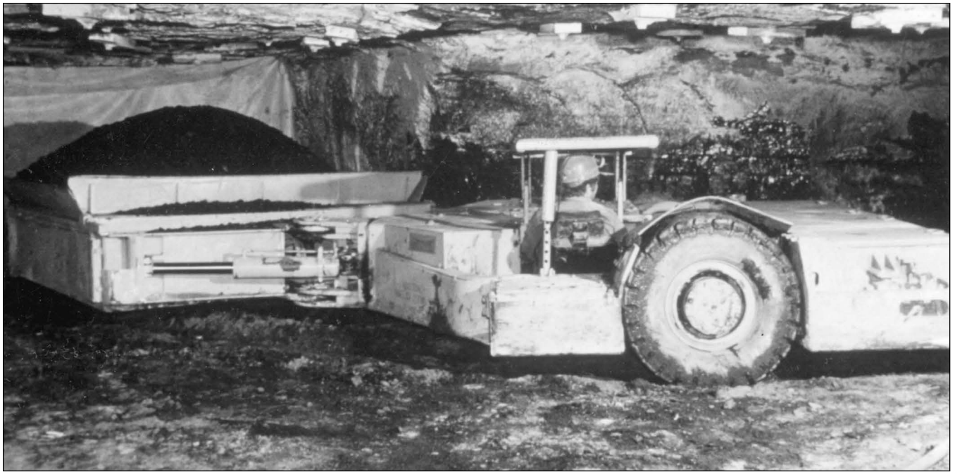
Figure 94 Mine and location unknown. Articulated shuttle car used for coal haulage from the continuous miner to the conveyor belt for transport out of the mine.
