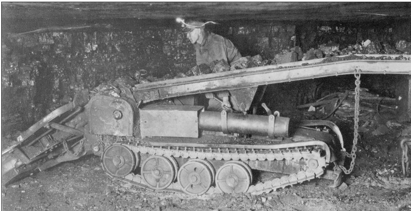
Figure 56 Bell & Zoller Coal Company, No. 2 Mine, Franklin County. An early Joy loader, moving on crawlers, vastly improved maneuverability and underscored the limitations of track haulage at the face (Ledvina et al. 1992).
