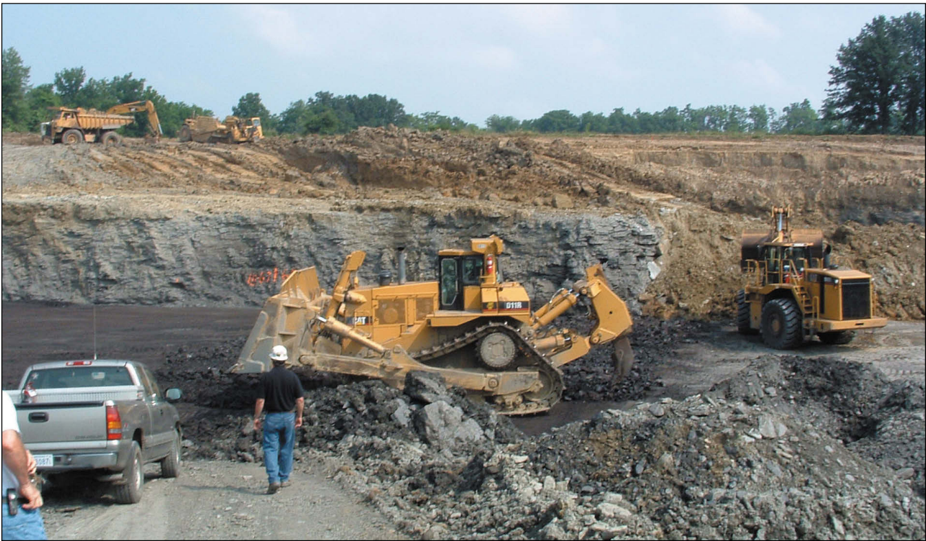
Figure 264 Vigo Coal Company, Wabash County. In current surface mining, the machines used look like machines at any construction site —shovels, trucks, and bulldozers. The equipment on the highwall is removing overburden without the aid of giant stripping shovels and draglines. The Caterpillar D11R in the foreground has a bulldozer blade on the front, and the rear has a tool to rip the coal into large blocks.
