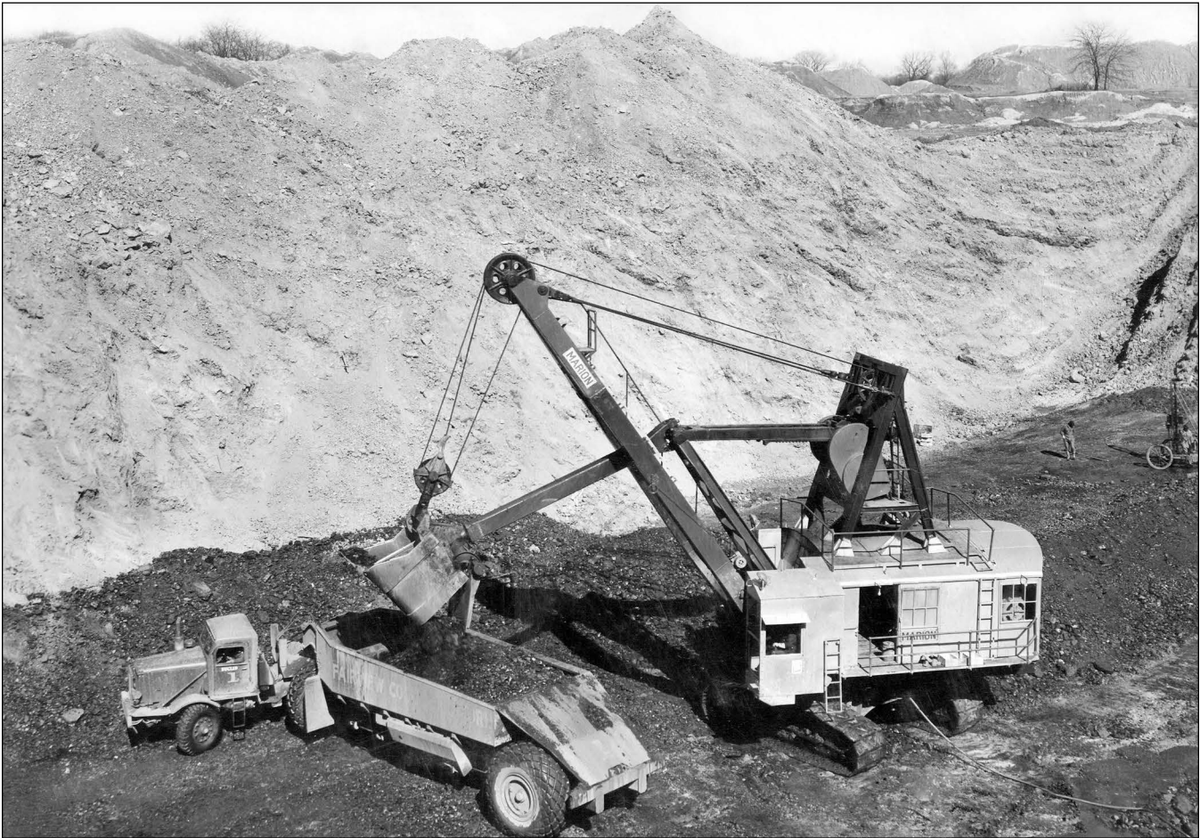
Figure 218 Fairview Collieries Corporation, Harmattan Mine, Vermilion County. A Marion Type 4121 shovel fills a Euclid coal hauler. This shovel was the only Marion loading shovel with a knee-action crowd (Historical Construction Equipment Association 2002).
