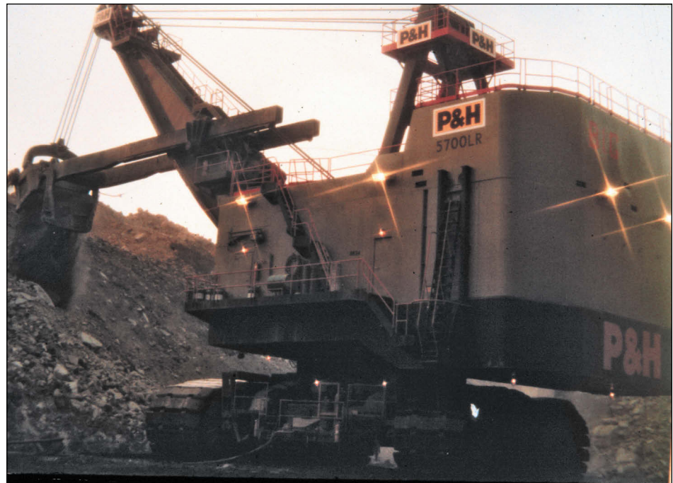
Figure 243 Southwestern Illinois Coal Corporation, Captain Mine, Perry County. This P&H 25-cubic yard shovel has twin dipper sticks to stabilize the bucket and keep it from twisting rather than the double hoisting rope system of larger shovels. The dual ropes here only hoist at the center of the bucket.
