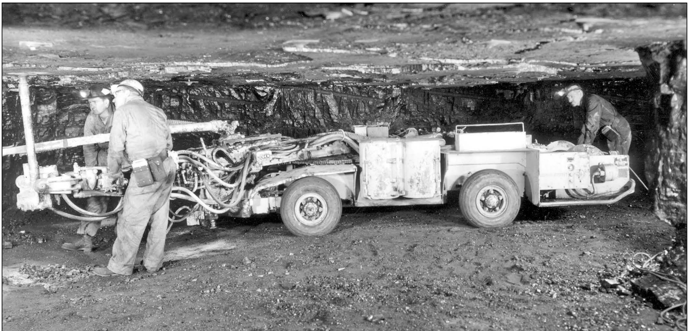
Figure 142 Mine and location unknown. The later roof bolting machines, such as this Jeffrey Model 261 in the 1950s, included an extendable boom (retracted in photograph) and remote operation (Ledvina et al. 1992).
