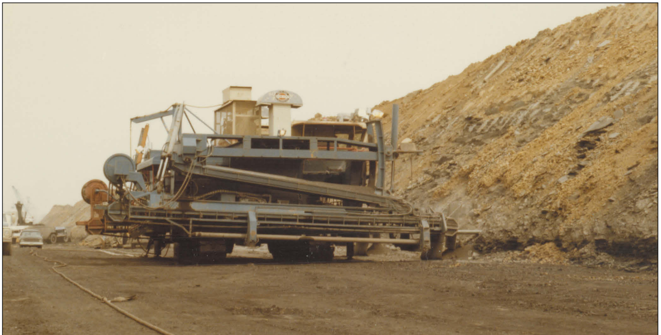
Figure 251 Arch of Illinois, Inc., Captain Mine, near Willisville, Perry County. Horizontal drill holes were often used to shoot the overburden from the coal in Illinois surface mining. At the Captain Mine, these holes were drilled 60 feet into the highwall about 3 feet above the Herrin Coal, ordinarily in the Brereton Limestone.
