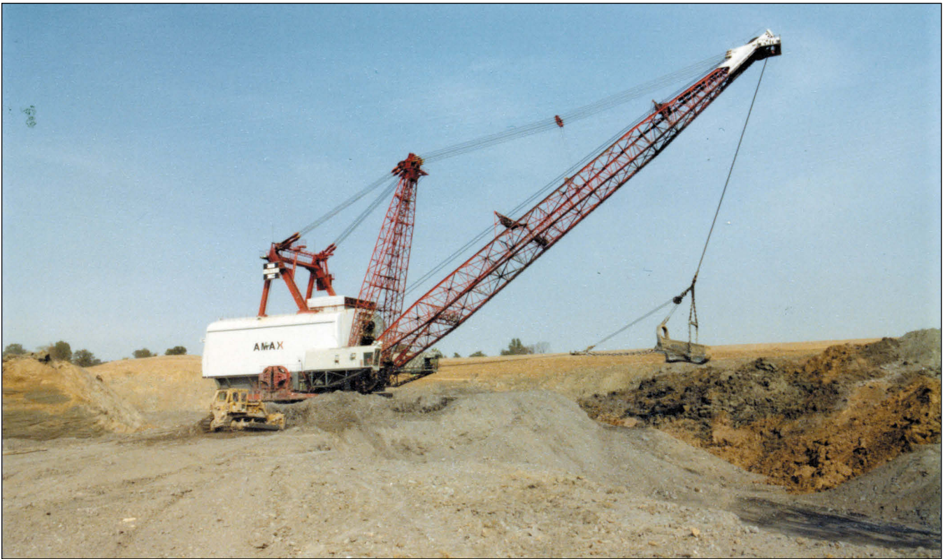
Figure 245 Amax Coal Company, Delta Mine, near Crab Orchard, Williamson County. A Bucyrus-Erie 1450-W walking dragline removing overburden. Amax reported that this machine had a 250-foot boom with a 60-cubic yard bucket.
