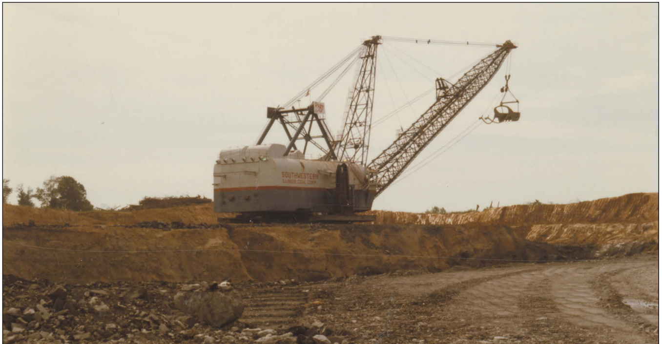
Figure 248 Arch of Illinois, Inc., Captain Mine, near Willisville, Perry County. A Page walking dragline with a 40-cubic yard bucket removing overburden.
