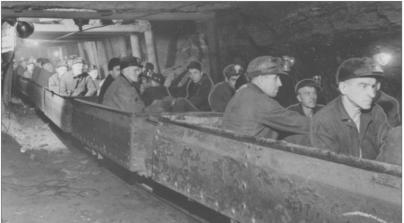
Figure 22 Zeigler Coal Company, mine and location unknown. Loaded mantrip departs for working sections. This photograph shows a full shift of miners and bosses ready to leave the shaft area for their working places inside the mine at the start of the shift. Note the open carbide lamps (Ledvina et al. 1992). Electric lamps were available in 1902, but were very heavy and not accepted by many miners (Crowell 1995). John E. Jones (1954), noted for rock dust research, indicated that closed lights of 1917 antagonized labor in a serious way, because the two-candle power lights were too dim to work by and were nicknamed “bug lights.” Later electric cap lamps with over 100-candle power bulbs and battery packs were comparatively light and much more acceptable to the men who had to use them. Such lights weighed about 6 ounces, and the battery pack weighed slightly less than 4 pounds, according to a 1942 advertisement for Wheat Lamp Sales. Flames were then present in the mines only behind the wire mesh of the safety lamp that was used to indicate the presence of methane or the lack of oxygen.
