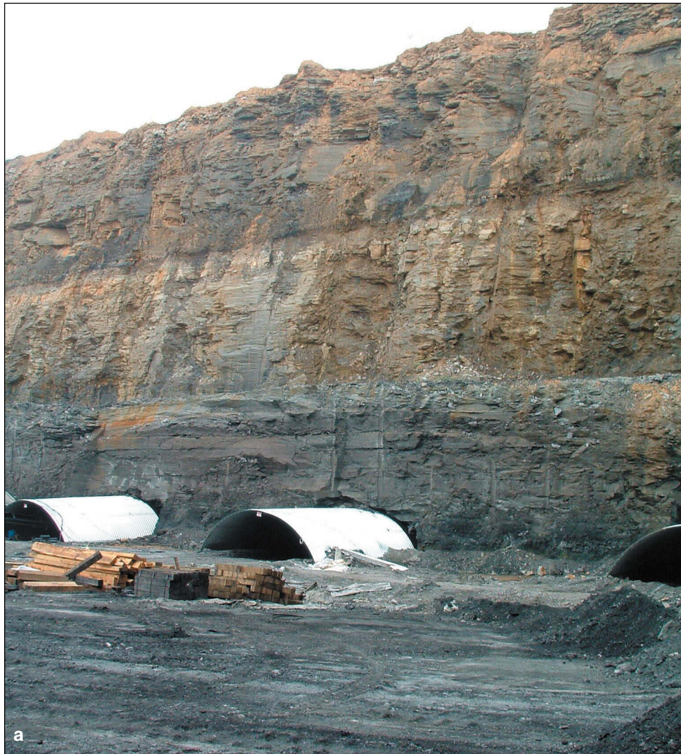
Figure 272 Illinois Fuels Company, LLC, I-1 Underground Mine, Saline County. The most common manner of accessing deep coal off the highwall in Illinois was to open a drift mine and work the coal in the usual underground mining pattern. The corrugated metal arches shown in the photographs protect people and equipment near the opening from rocks falling from the highwall. Photograph (b) shows the conveyor carrying the mined coal out of the mine.
