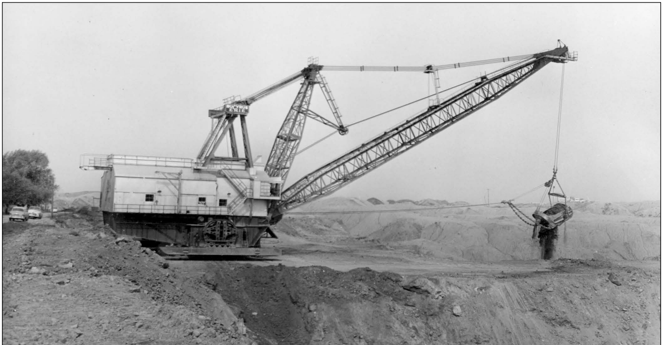
Figure 216 Fairview Collieries Corporation, Harmattan Mine, Vermilion County. This Bucyrus-Erie 1150 walking dragline from 1949 has a 25-cubic yard bucket on a 180-foot boom (Hollingsworth 1963). An advertisement for the machine offered a version with a 250-foot boom, although with a smaller bucket size.
