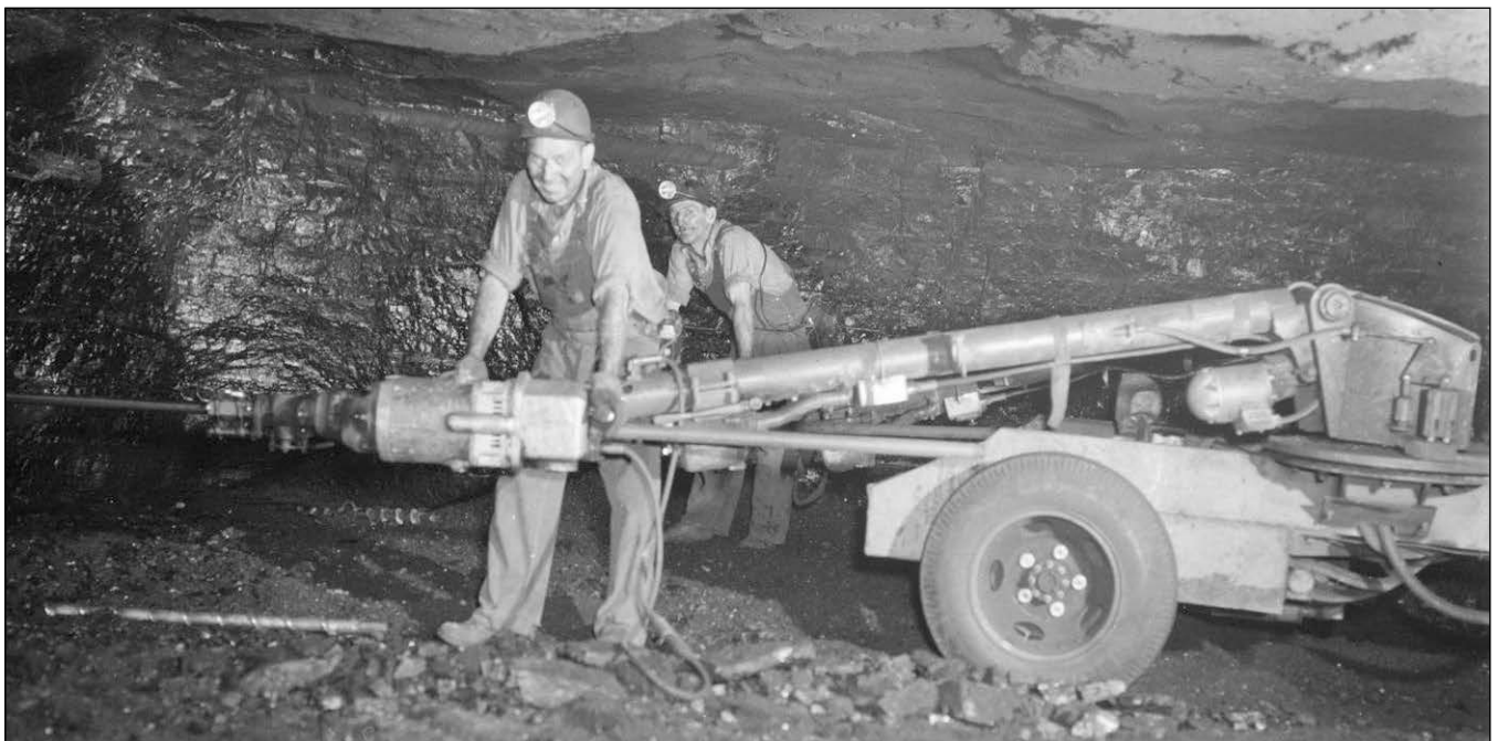
Figure 40 Peabody Coal Company, mine and location unknown. Automatic drills such as the one shown in the photograph vastly improved drilling speed and efficiency.
