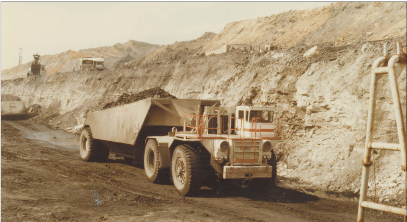
Figure 261 Arch of Illinois, Inc., Captain Mine, near Willisville, Perry County. The Captain Mine generally used 120- to 150-ton capacity haulage trucks, such as this Rimpull hauler.
