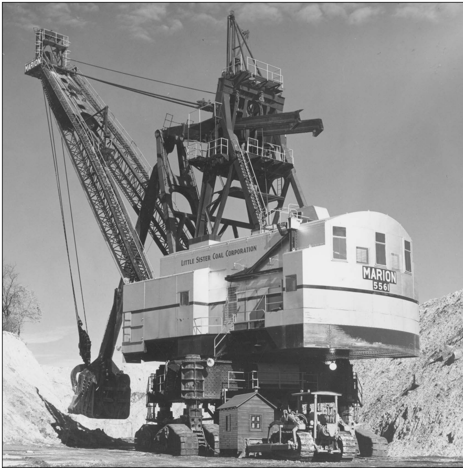
Figure 219 Little Sister Coal Corporation, Little Sister Mine, Fulton County. This Marion 5561 stripping shovel towers over the pit. The shovel had a 35-cubic yard bucket and weighed 1,675 tons. This shovel, introduced in 1940, was the first Marion shovel with the knee-action crowd (Historical Construction Equipment Association 2002).
