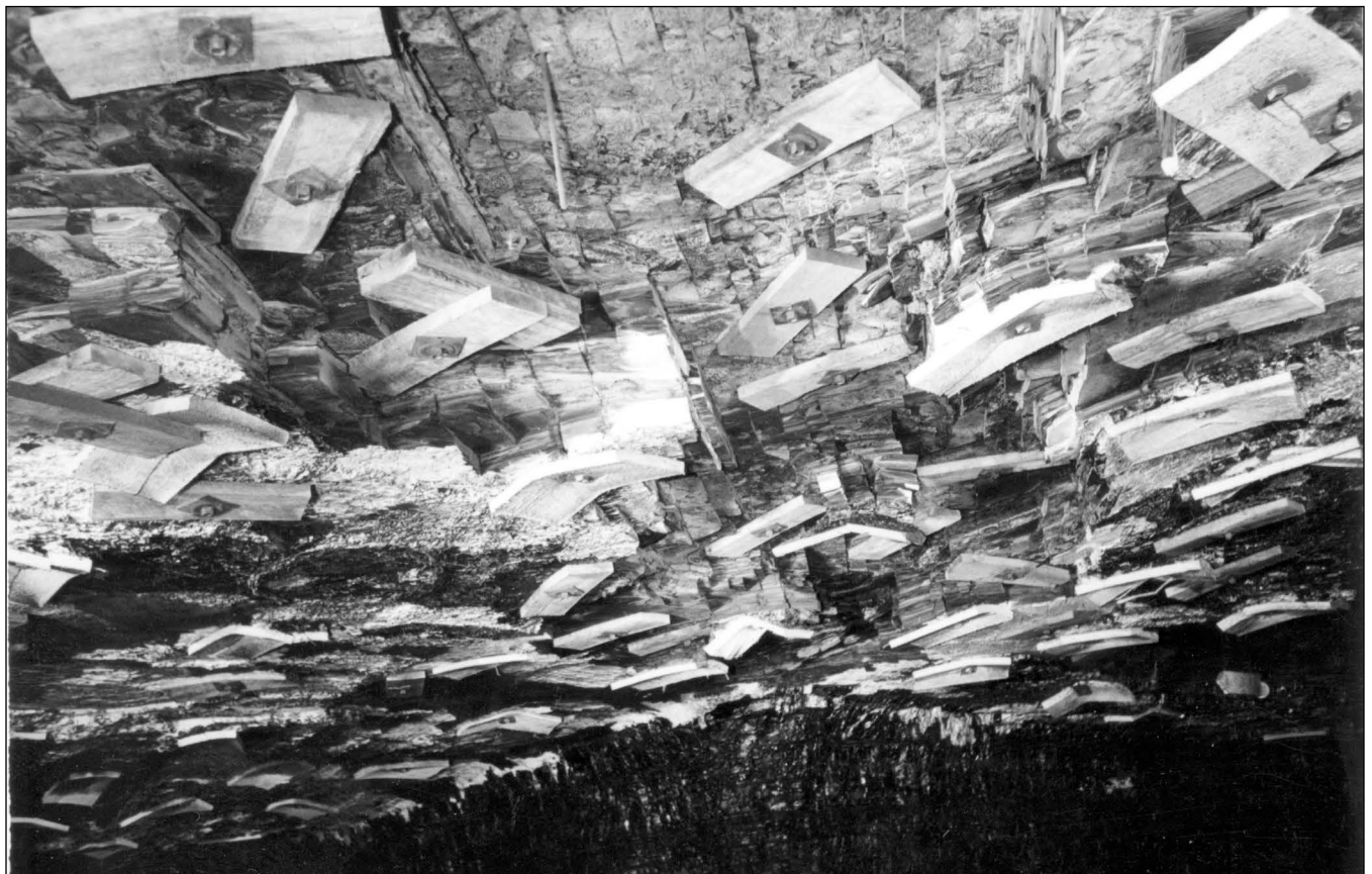
Figure 138 Peabody Coal Company, No. 10 Mine, in Christian County. The black shale roof required heavy bolting because of the closely spaced joints (fractures) in the shale. As the roof-bolting process matured, resin-anchored head rebar roof bolts became the most commonly used in U.S. coal mines, followed by standard mechanical roof bolts (Scott 1989). Specialty bolts are used less frequently, and such bolts are generally mechanically anchored bolts that have resin enhancements in the fixtures (Scott 1989).
