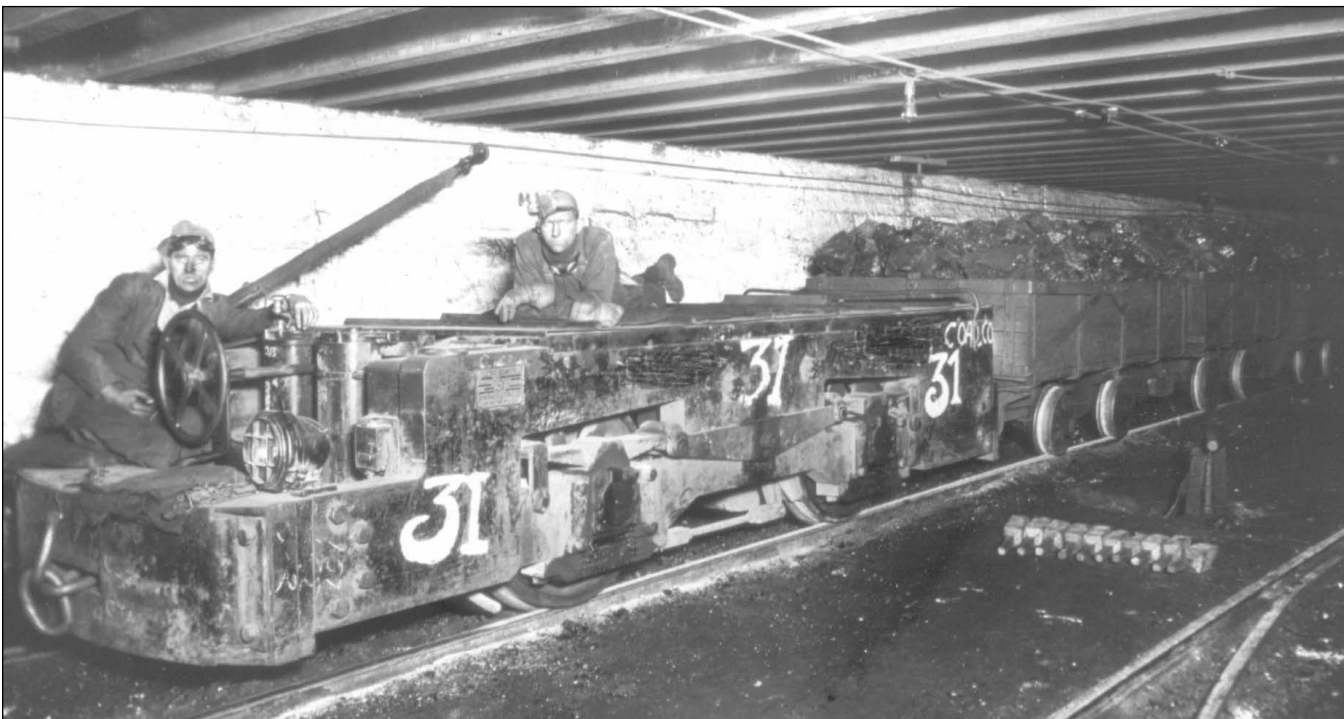
Figure 69 Mine and location unknown. An electrical trolley engine with a loaded trip of coal cars, operator, and assistant. The connection to the trolley wire is by a spring-loaded pole. An uneven roadbed could shake the pole loose from the connection (W. John Nelson, personal communication).
