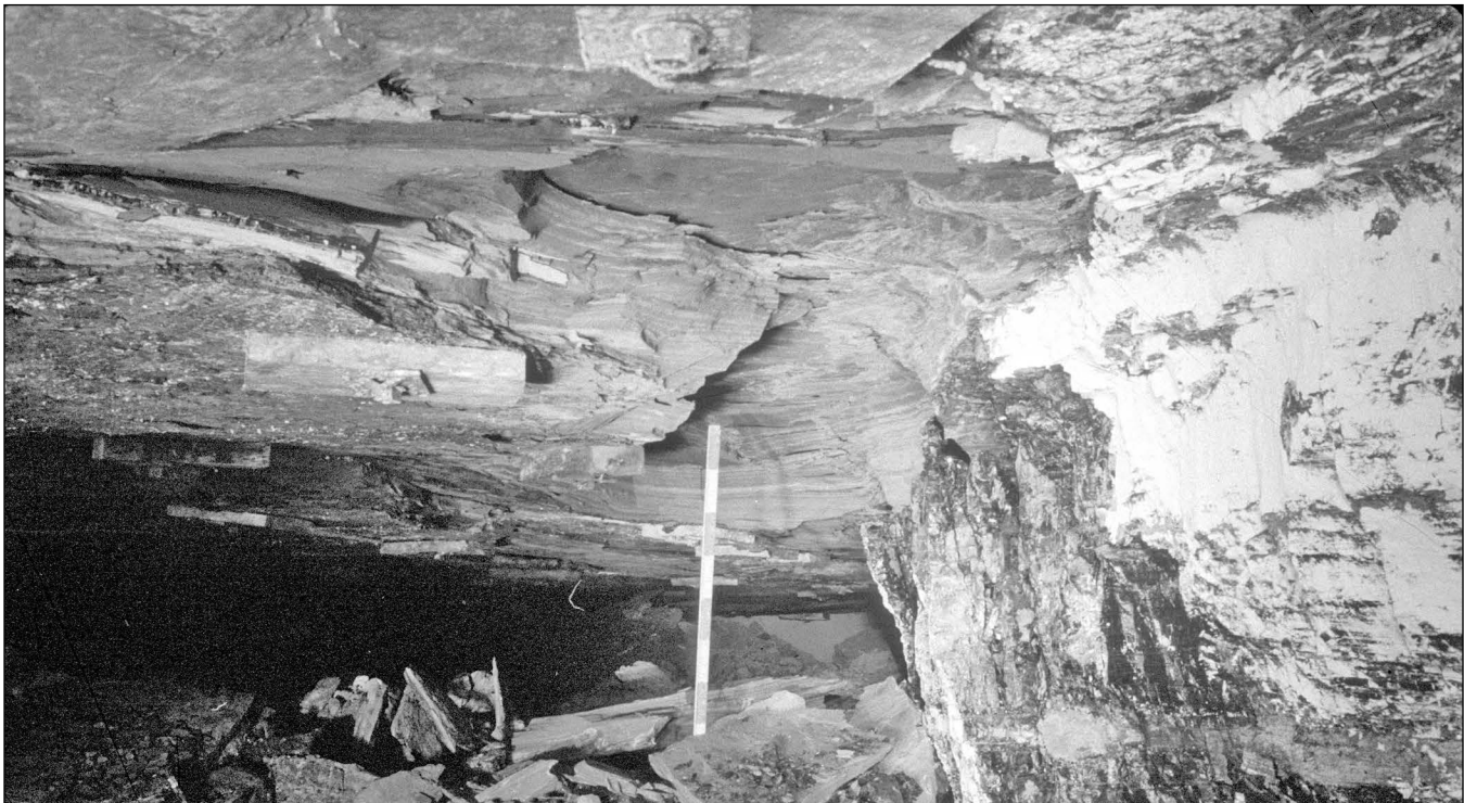
Figure 144 Hillsboro Mine, Montgomery County. Even when the roof has been bolted, weathering, jointing, and other stresses can combine to cause slabs of the roof to come down (Pitts 1939).
