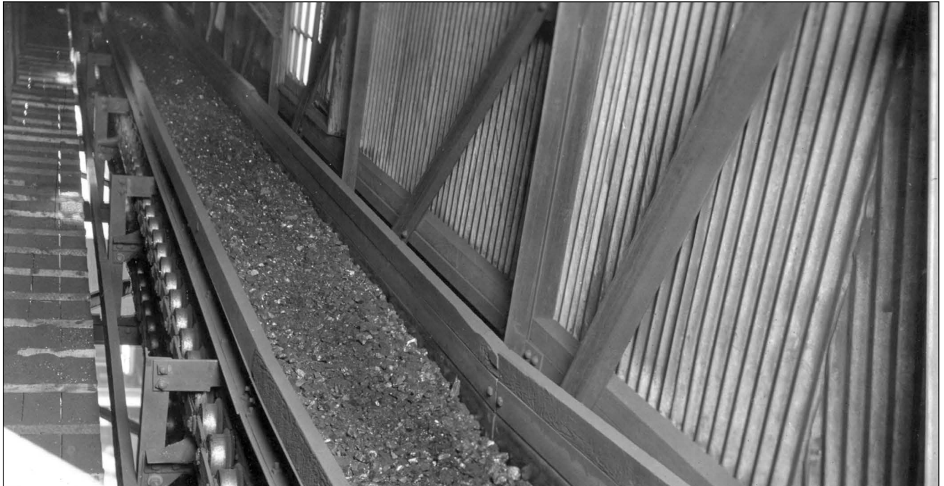
Figure 105 Big Creek Coals, Inc., No. 4 Mine, Saline County. Early conveyor systems had wooden sides to keep the coal on the belt. Later conveyors had shaker systems that distributed the load more evenly and a trough shape that kept the coal in the center of the belt.
