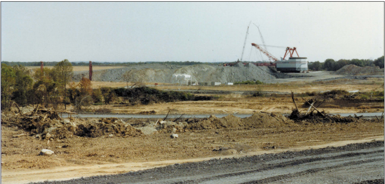
Figure 246 Amax Coal Company, Delta Mine, near Harco, Williamson County. A Bucyrus-Erie 3270-W walking dragline under construction towers over the surrounding countryside. The boom, still horizontal and supported by earth at this point of assembly, was 330 feet long. When the dragline was completed, the bucket held 176 cubic yards. The completed machine weighed 8,750 tons. Amax purchased the only two of these machines made, and they are still the second largest draglines ever built (Haddock 2001).
