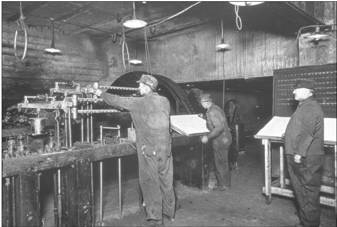
Figure 107 Mine and location unknown. These men are weighing and recording the coal production prior to hoisting or dumping the coal. This mine appears to have a rotary dump similar to that shown in Figure 109.
