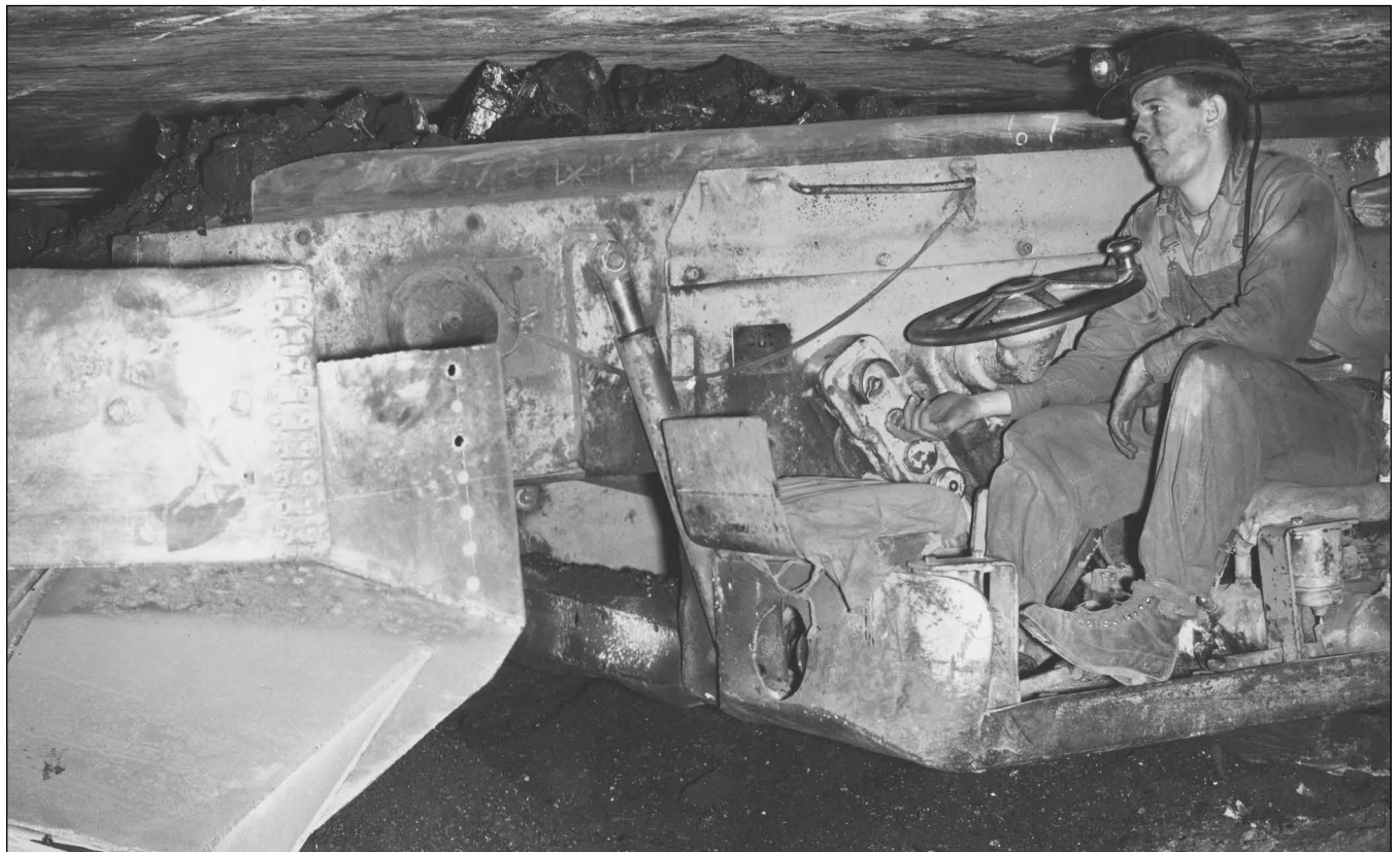
Figure 75 Sahara Coal Company, No. 5 Mine, Saline County. The operator is discharging coal from the shuttle buggy into the transfer pickup to the left that, in turn, loads coal on the rubber belt (Ledvina et al. 1992).
