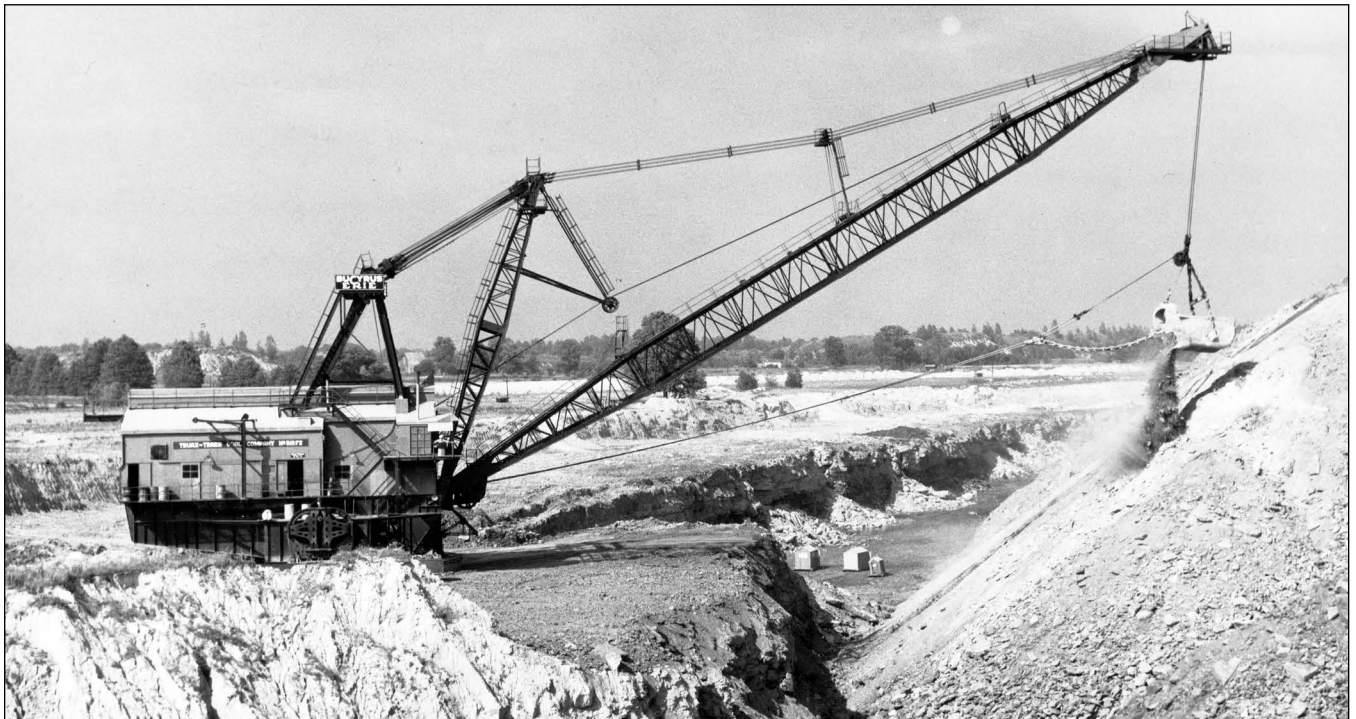
Figure 220 (below) Truax-Traer Coal Company, Burning Star Mine, near DeSoto, Jackson County. This Bucyrus-Erie walking dragline, probably an 1150-B, deposits spoil from the highwall to the other side of the pit (Ledvina et al. 1992). The 20-cubic yard bucket on a boom about 200 feet long did its job very well. This machine weighed 1,265 tons (Haddock 2001).
