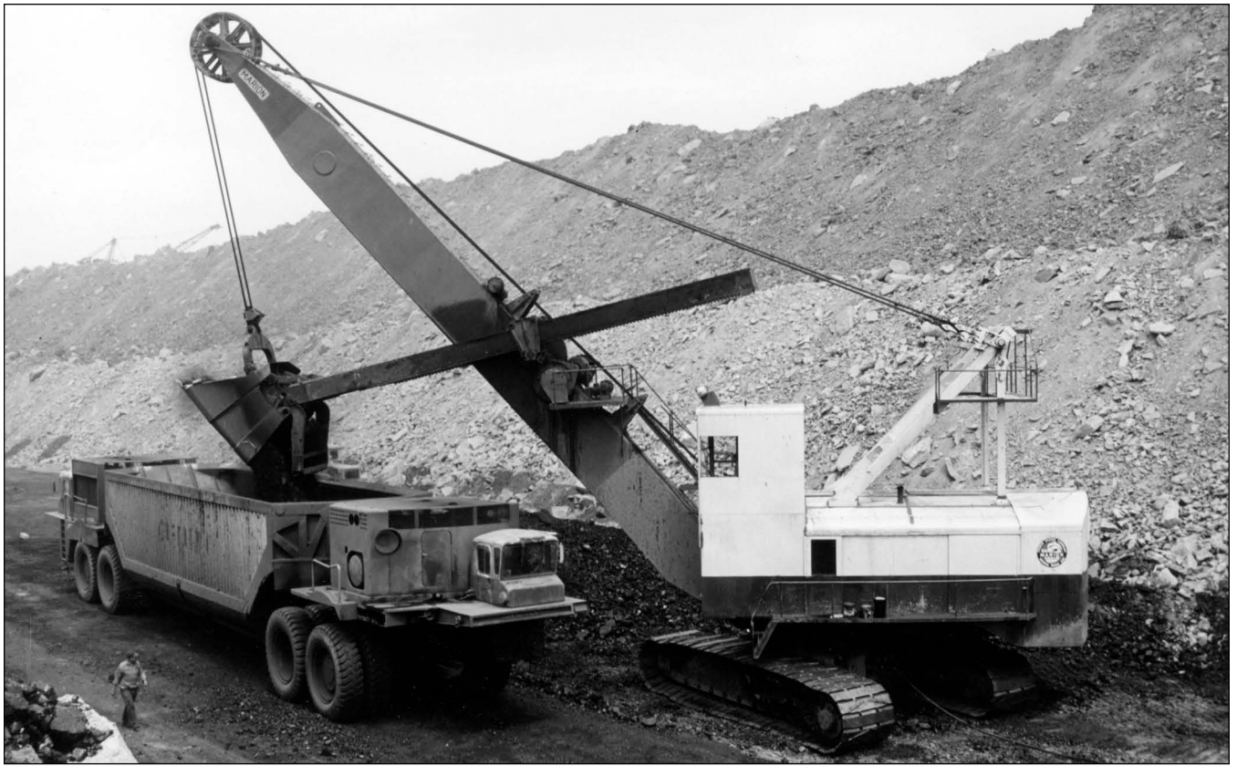
Figure 232 Southwestern Illinois Coal Corporation, Captain Mine, near Willisville, Perry County. This 240-cubic yard truck is being filled by a Marion loading shovel. Cabs in both front and back of the truck mean that the awkward vehicle does not have to be turned around, which could save considerable time in the confines of a narrow pit or loading facility.
