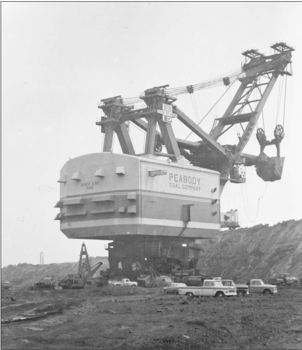
Figure 234 Peabody Coal Company, River King Mine, near Freeburg, St. Clair County. This Bucyrus-Erie 3850-B stripping shovel was a heavier version of the same model constructed for Peabody's Sinclair Mine in Kentucky. It had a 200-foot boom for a 140-cubic yard bucket and weighed 9,350 tons. The parts came from the Bucyrus-Erie plant in South Milwaukee on 300 railcars. When the shovel was decommissioned in 1992, the operator, Jim Paglia, was the same man who began its career in August 1964 (Haddock 2001).
