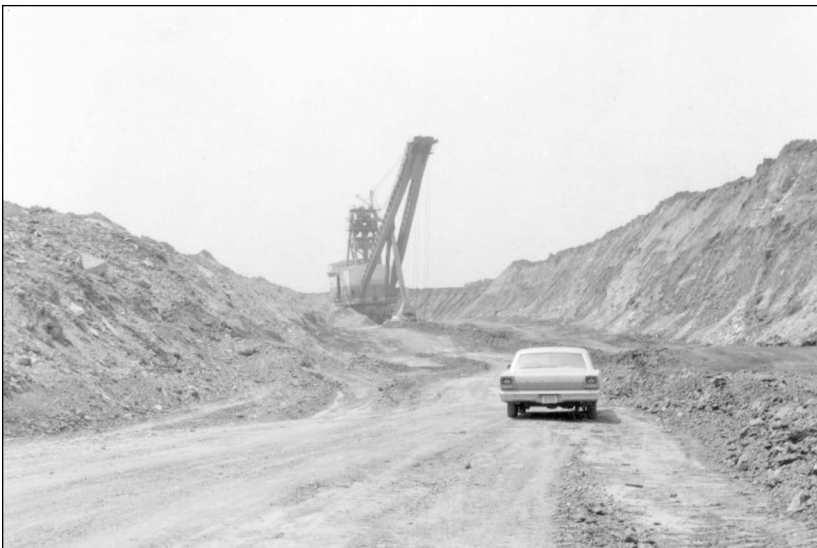
Figure 235 Midland Electric Coal Company, Elm Mine, near Victoria, Knox County. The shovel in the background is a Marion 5760 with a 60-cubic yard bucket (Historical Construction Equipment Association 2002). This model is the same as the famous shovel, "The Mountaineer," which operated in Ohio and had a 65-cubic yard bucket. The Mountaineer, built in 1955, had the first elevator for the operators (Haddock 2001). This safety feature was installed on all large shovels afterward so personnel could get to the revolving upper frame from the stationary lower frame without accident.
