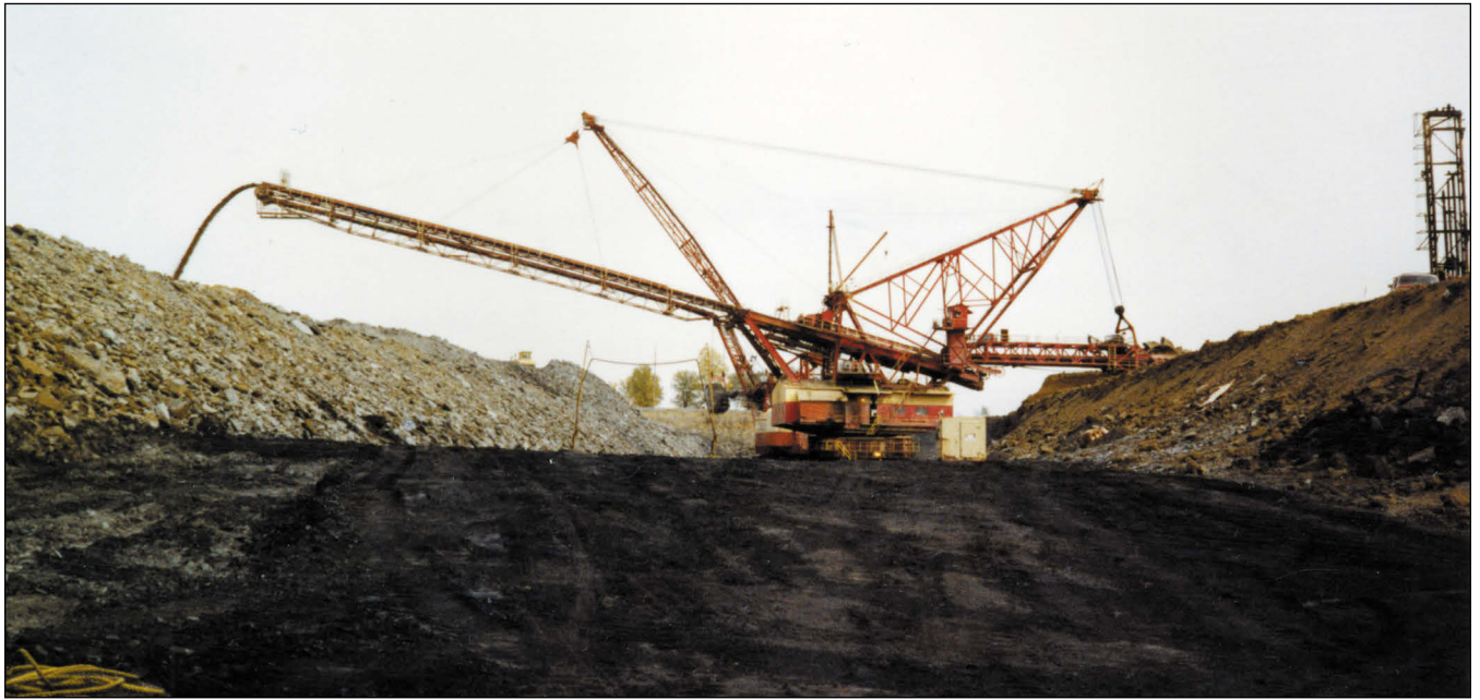
Figure 262 Freeman United Coal Companies, Industry Mine, McDonough County. This 2,000-ton bucket wheel excavator removed subsoil and deposited it directly onto the rock spoil pile for reclamation. The Industry Mine collected the topsoil into piles with bulldozers and scrapers and moved the topsoil piles with the bucket wheel excavator as well. This process avoided excessive rehandling of the topsoil material. In 1993, yields on reclaimed prime farm land exceeded requirements. This bucket wheel excavator was still operating in 2003 and was the last operating bucket wheel excavator in the United States. At the far right, a vertical drill made holes for blasting on the part of the highwall that had subsoil removed.
