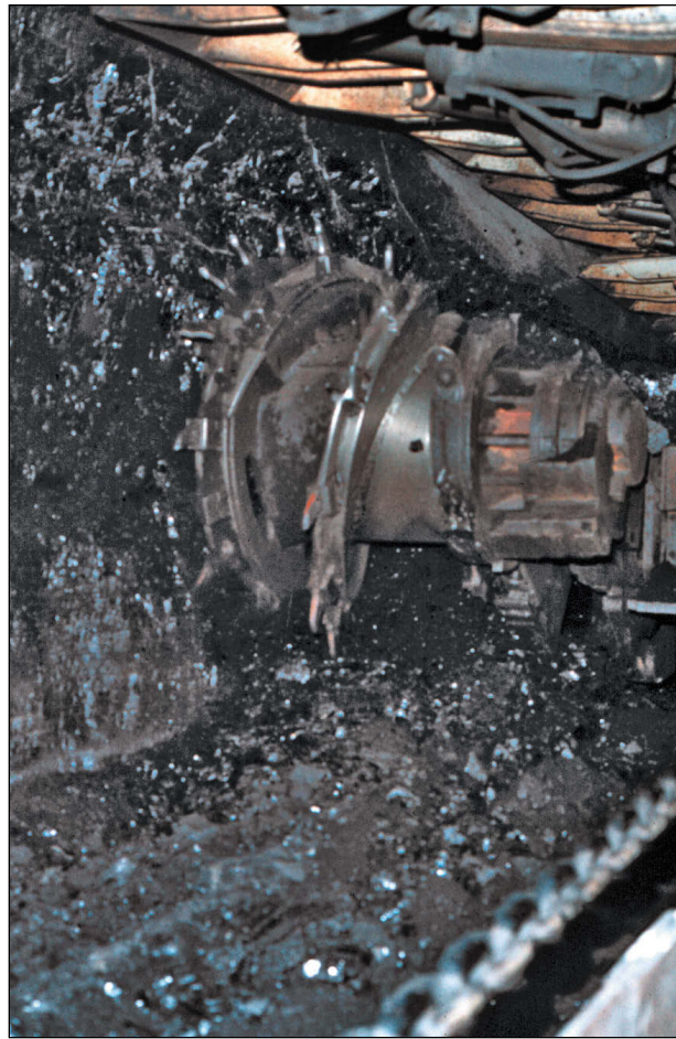
Figure 96 Old Ben Coal Corporation, mine and location unknown. The cutting bit of a drum shearer longwall installation is shown in this photograph. The coal is to the left, and the unit advances to the left after the cutter travels the length of the panel. The mined coal drops to a chain conveyor, where it is transported to the secondary conveyor haulage and then to the main conveyor.
