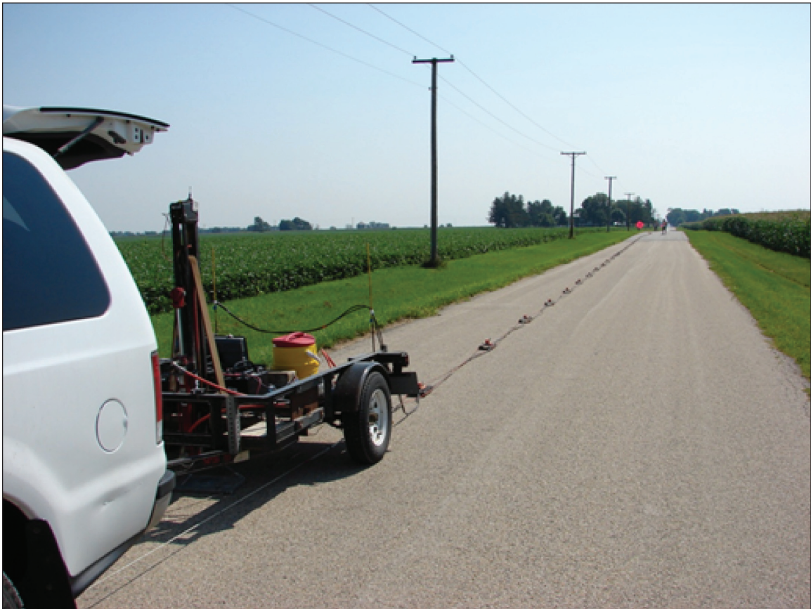
Figure A1 Photo showing the acquisition process of the P-wave seismic reflection data. The long land streamer and the weight drop are towed by a car along the survey line, while data were acquired at 13 foot intervals along the line.
