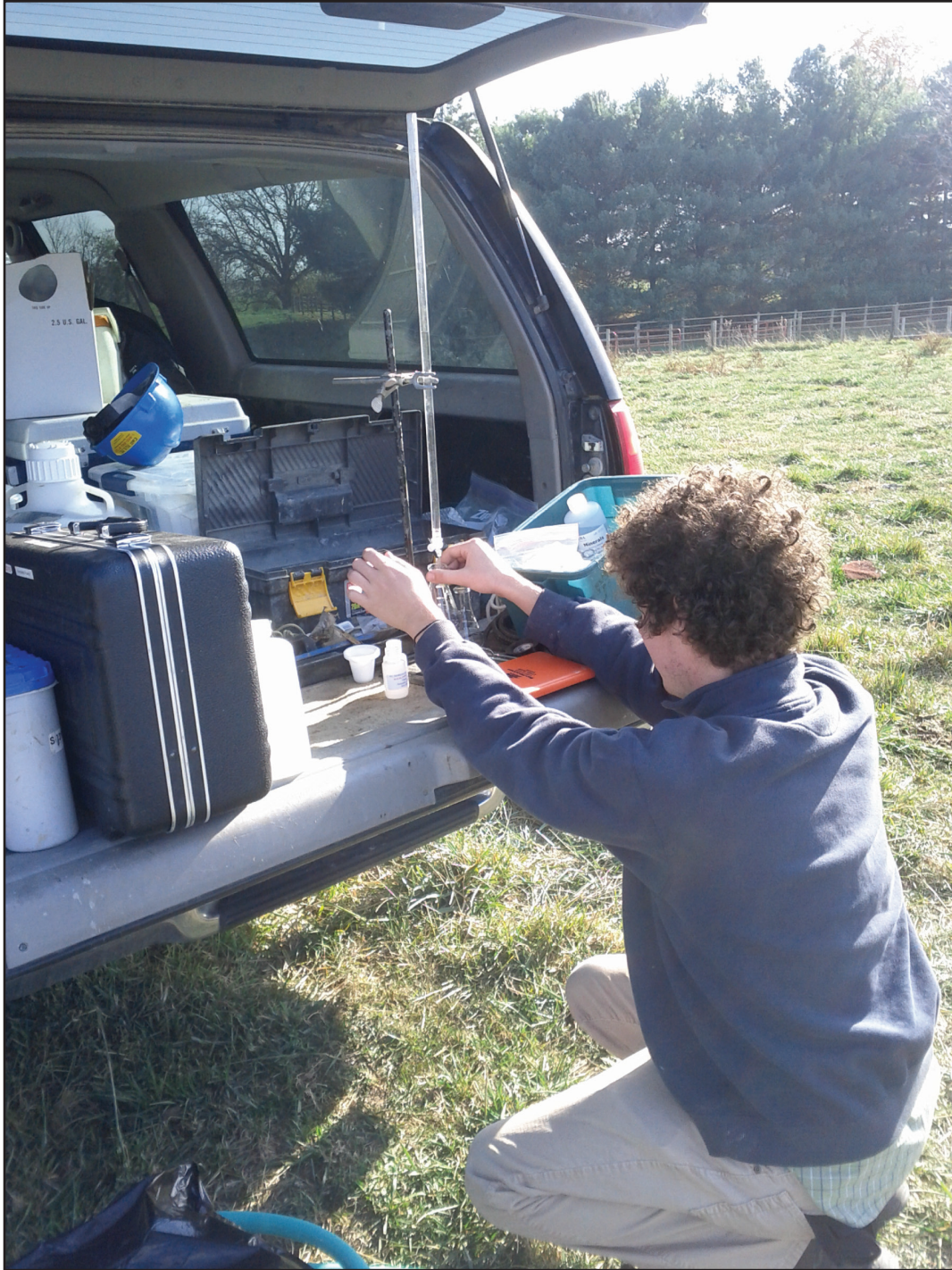
Figure 6 Determination of alkalinity in groundwater samples using titration technique.
