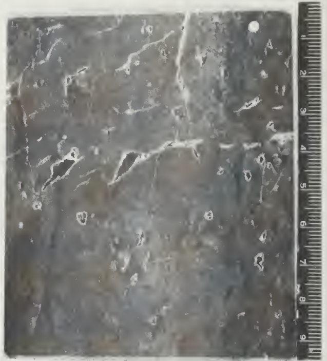
Fig. 5 - Polished core of Shakopee Dolomite (at depth of 9,669 feet) taken from the Texaco No. 1 Cuppy, Hamilton County, Illinois (hole 4 of this report). Porosity can be seen in the form of vugs (black areas) and fractures (white lines). (The straight vertical line in the lower left quadrant of the core is a scratch on the core.) Scale is in centimeters.
