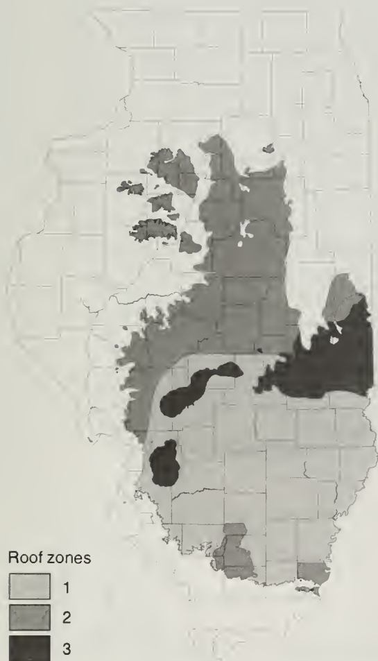
Figure 20 Zones used to assign minimum thickness of bedrock overburden for underground mining of the Herrin Coal.
