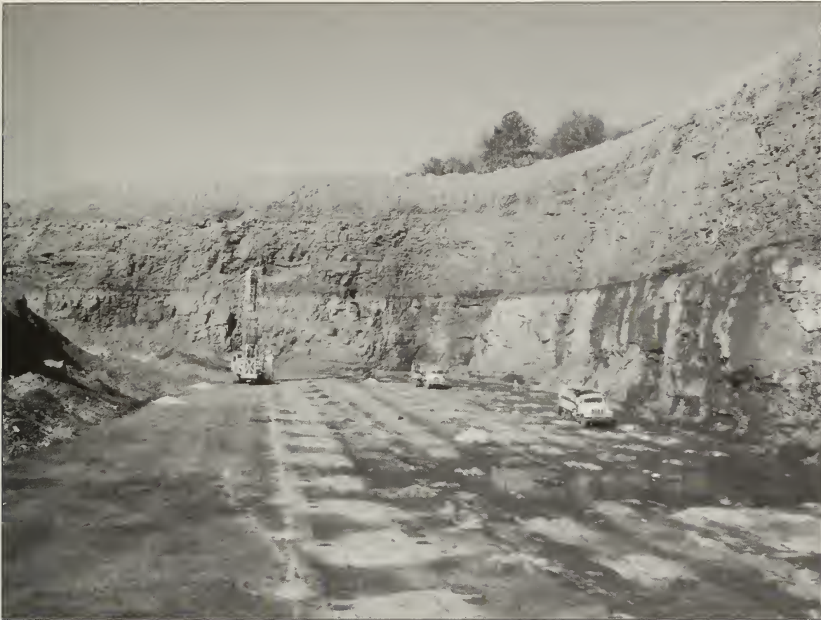
Figure 21 Stop 4: Surface mining pit at Jader Coal Company (photo by R.J. Jacobson). A view looking west in one of the pits of Jader Coal Company. At the base of the highwall to the right of trucks is the Dekoven Coal, which has been removed in this cut. The drill rig is making holes for placement of explosive that will loosen the exposed strata below the Dekoven so that the Davis Coal (about 20–30 feet below the Dekoven Coal) may be mined.
