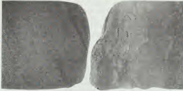
Figure 10c The lower core is a heavily bioturbated sand and shale mixture that is capped by a well laminated, green shale. The upper core is a clean, cross laminated sandstone. The sample is from Sanders No. 9 well (depth 2,163 ft).
