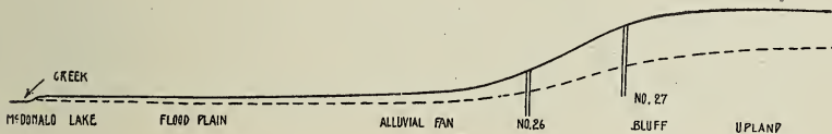
FIG. 9. Profile across upland bluffs one mile south of Peters, showing surface of ground water in relation to topography.
