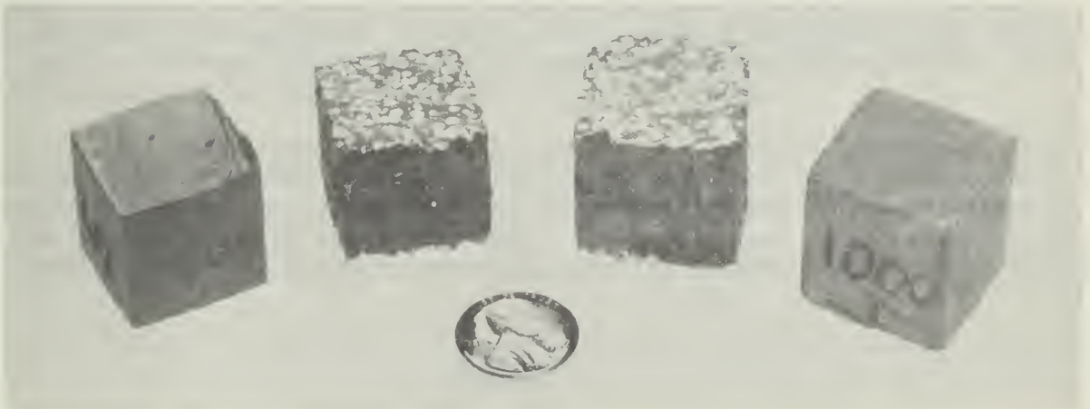
BRICK SPECIMENS MADE WITH RED-BURNING CLAY AND POLYSTYRENE BEADS (Holes in top surface of center pair of blocks have been filled with plaster of paris.)
