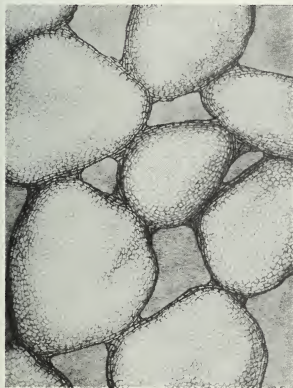
Figure 11. Sketch on Left of Montmorillonite Clay-Bonded Sand to Illustrate the Smooth Even Coating of Quartz Grains with Montmorillonite Flakes. Sketch on Right of Kaolinite Clay-Bonded Sand to Illustrate the Irregular Coating of Quartz Grains with Small Flakes and Large Lumps of Flakes. Based on Microscopic Examinations. (After Grim and Cuthbert)
