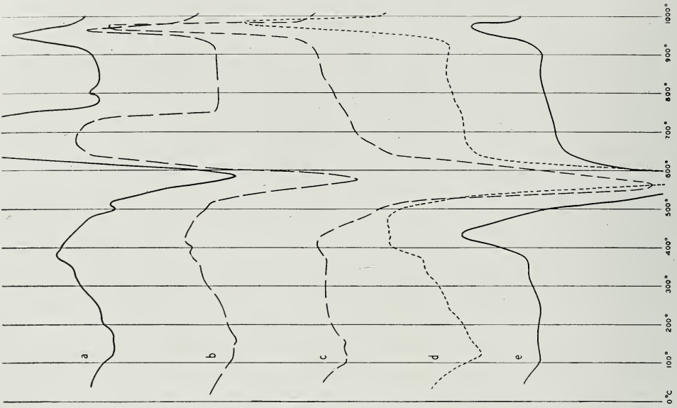
FIG. 14.—Samples of fire clay from clay pit of refractory plant, northern Ill., scale B (scale on Fig. 3).
