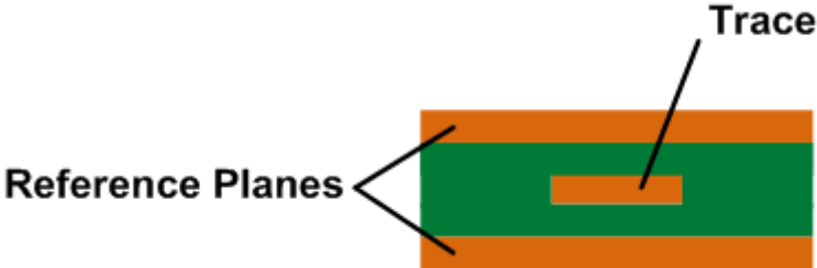
Figure 1.4: Stripline cross section.
