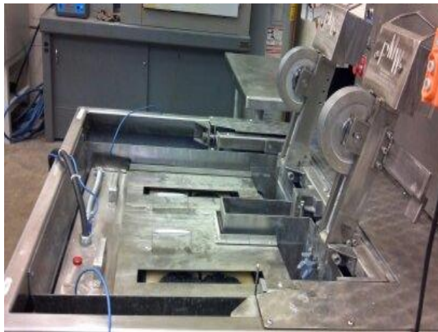
Figure 4.2. Hamburg loaded-wheel track test setup under dry and heated conditions.
