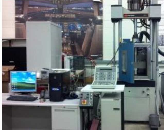
Figure 4.5. Test device used for the indirect tensile test, manufactured by Instron, Inc.
