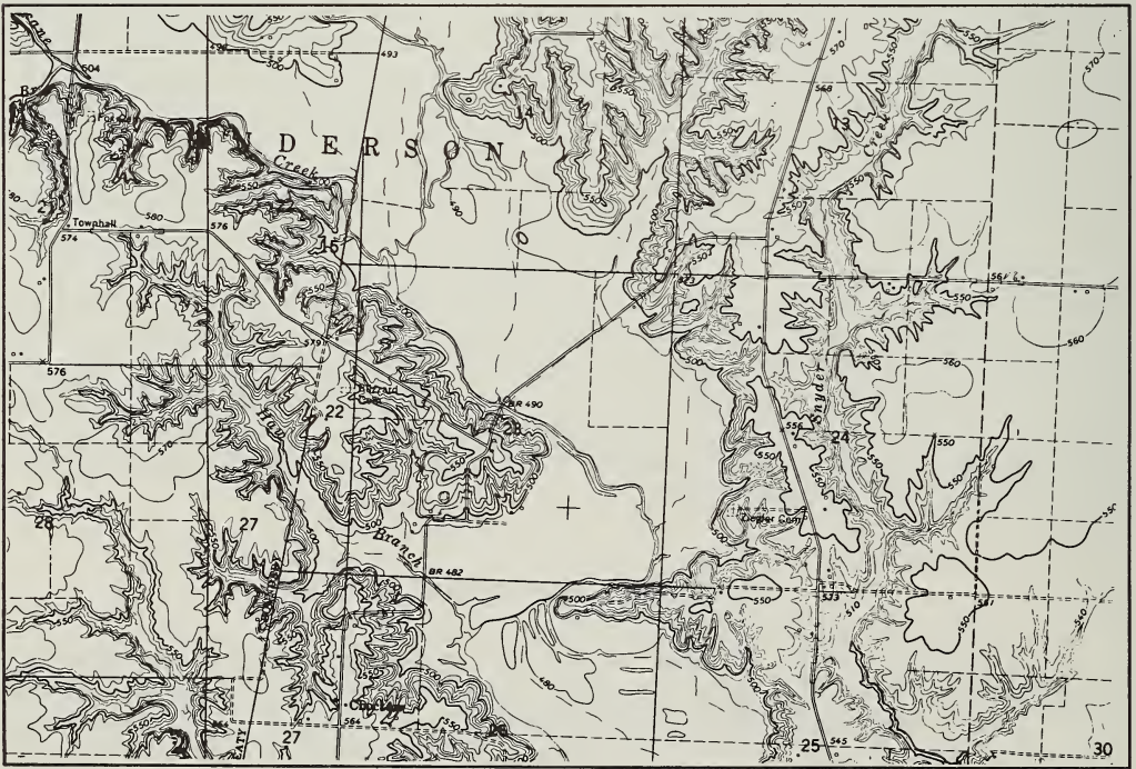
Fig. 6 - Maps of a portion of Clark County showing sections offset along Indian Treaty Boundary.
