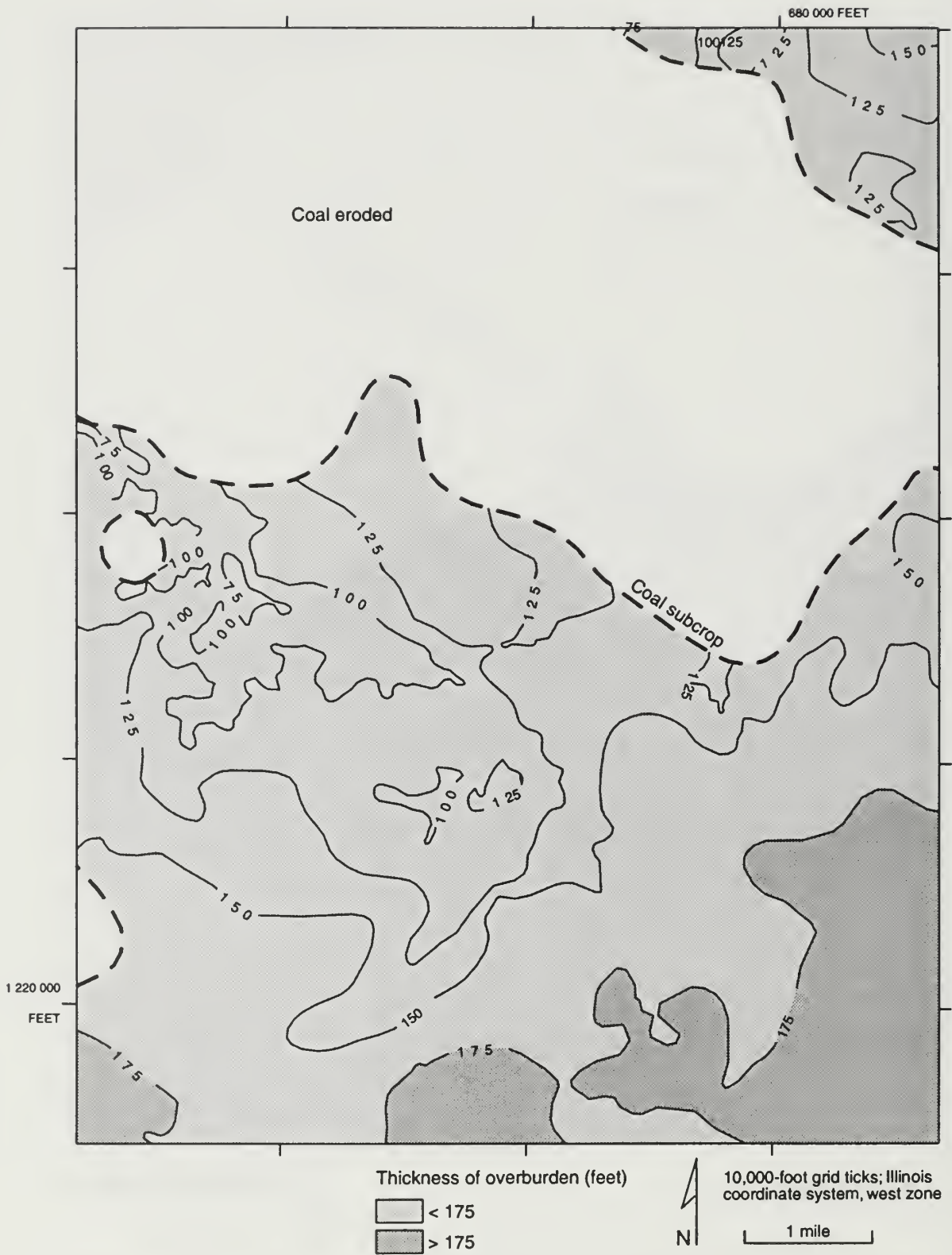
Figure 24 Thickness of overburden of the Danville Coal in the Middlestown Quadrangle. Contour interval is 25 feet.
