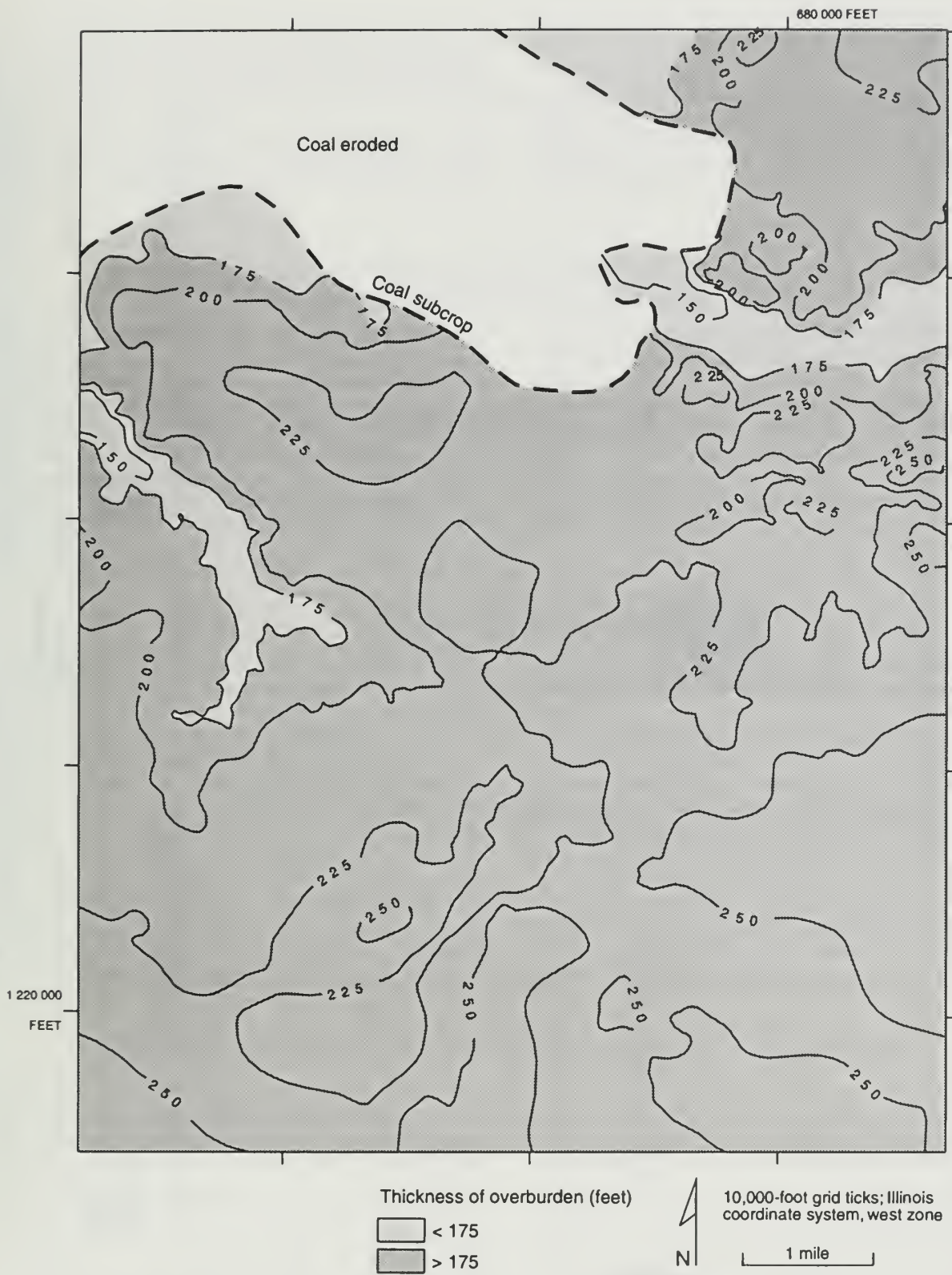
Figure 28 Thickness of overburden of the Springfield Coal in the Middletown Quadrangle. Contour interval is 25 feet.
