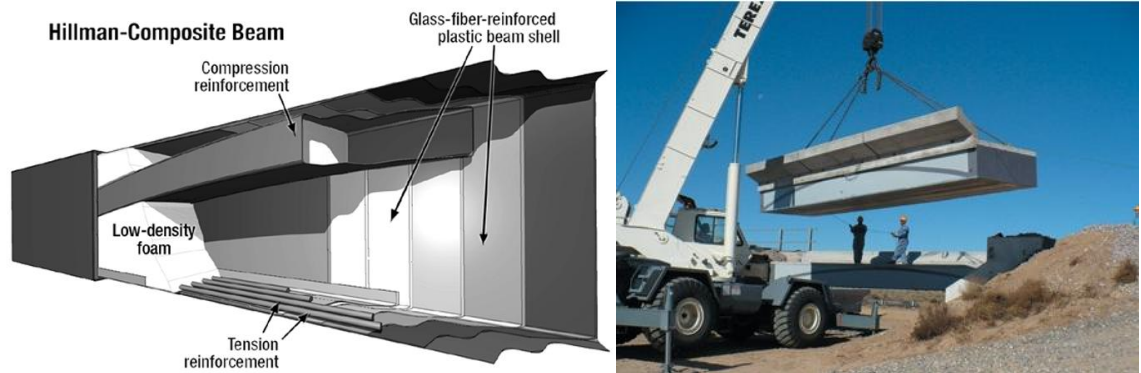
Figure 6.2. HC Bridge Company diagram (L) and product (R) while erected in Pueblo, Colorado (courtesy of HC Bridge Company, LLC).
