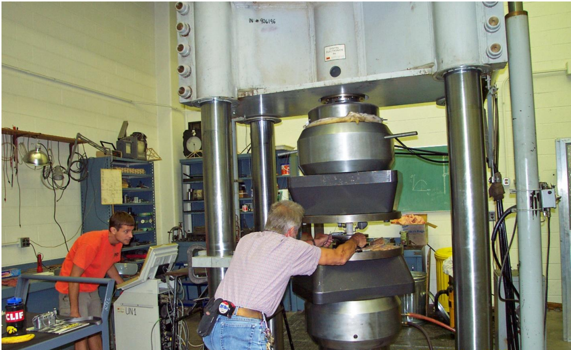
Figure 5.4. Concrete samples testing in the laboratory for a Class I railroad to validate concrete repairs in the field.
