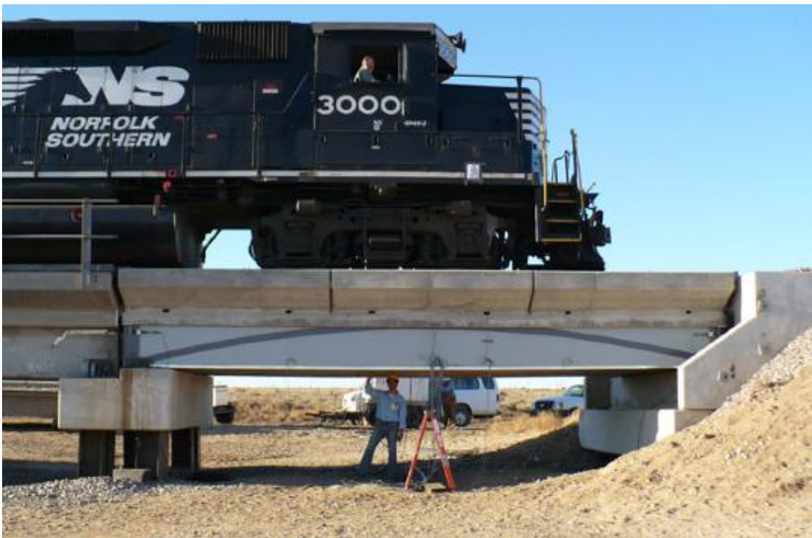
Figure 6.1. John Hilman showing his Hilman beam under railroad traffic at FAST (Pueblo, Colorado) (Courtesy of HC Bridge Company).
