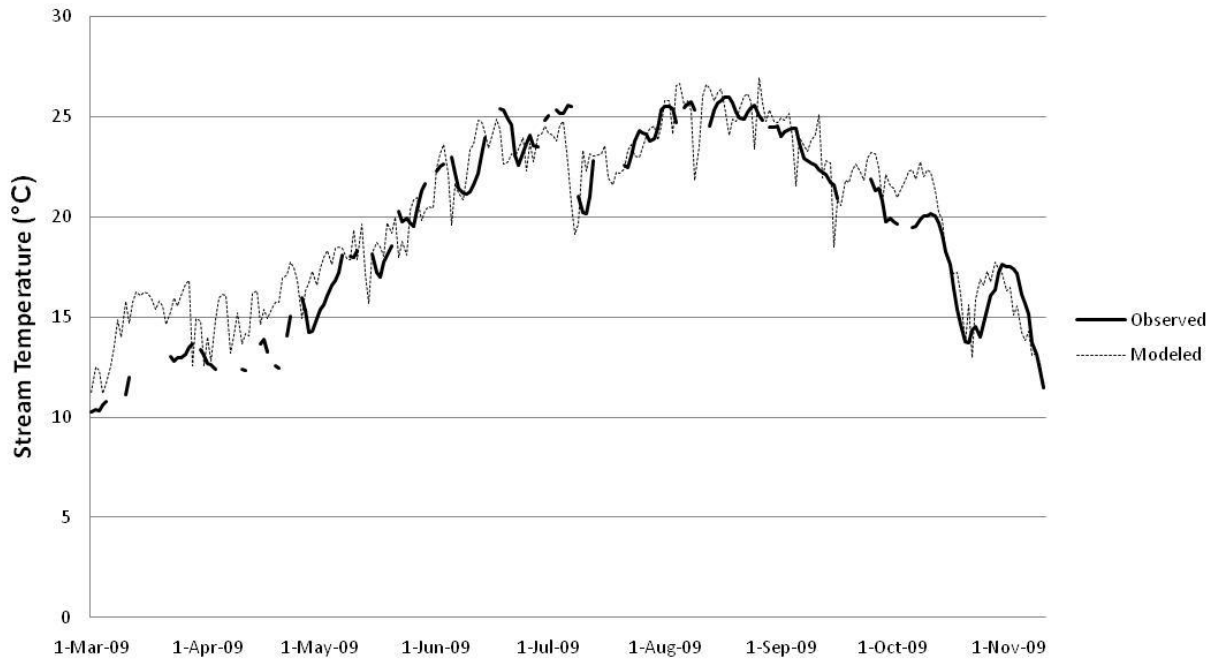
Figure 4.3 Observed and predicted temperature values for the Llobregat River during the warmer months of 2009 in which EDR modules are in operation at the drinking water facility.
