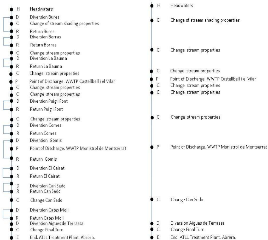
Figure K.1 A schematic representation of the complete and simplified Stream Network Model between the headwaters in Castellbell i el Vilar to the ATLL Water Treatment Plant in Abrera.
