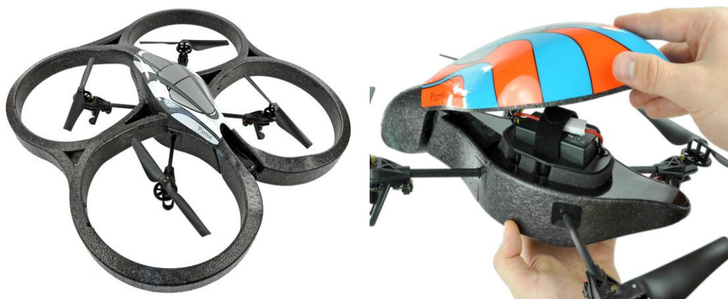
Figure 1.3 AR.Drone Appearance and the Interior Layout
