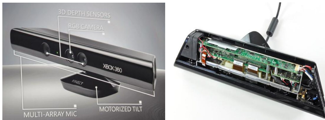
Figure 1.4 Kinect Appearance and Interior Layout
