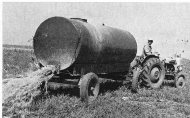
A 1,000-gallon tank wagon without agitator. Front of tank is 6 inches higher than rear. Manure spreads about 6 feet. (Fig. 15)
