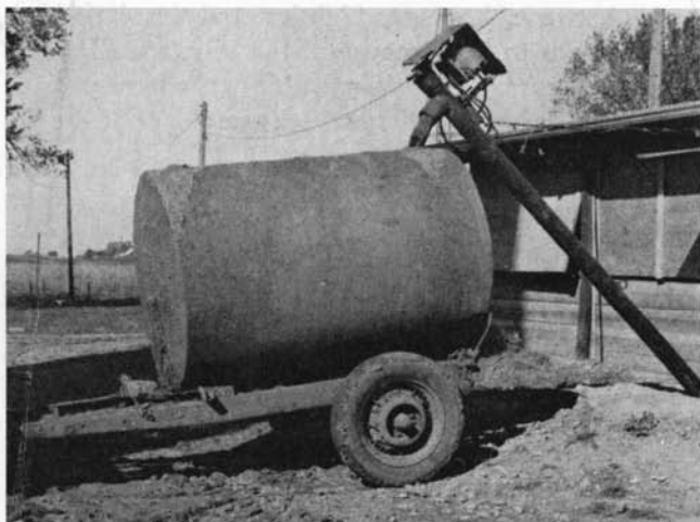
A 500-gallon tank wagon without agitator being filled with auger pump. (Fig. 14)
