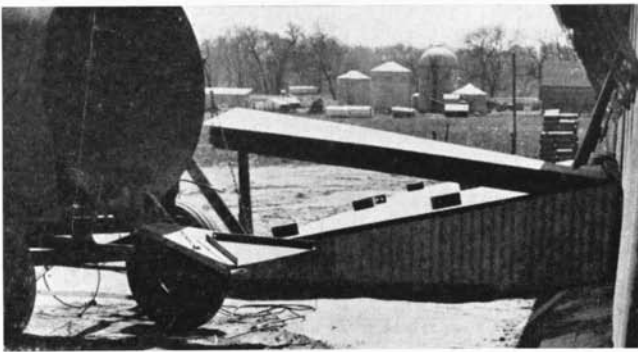
Wood and sheet-metal cover for 8-foot-wide storage tank. Note hinged section for inspection and clean-out. (Fig. 4)
