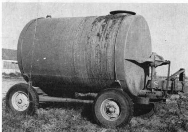
A 1,000-gallon tank wagon with "fan" spreader driven by tractor power take-off through auto differential. Auger through bottom of tank serves as drive shaft as well as tank cleaner. (Fig. 13)
