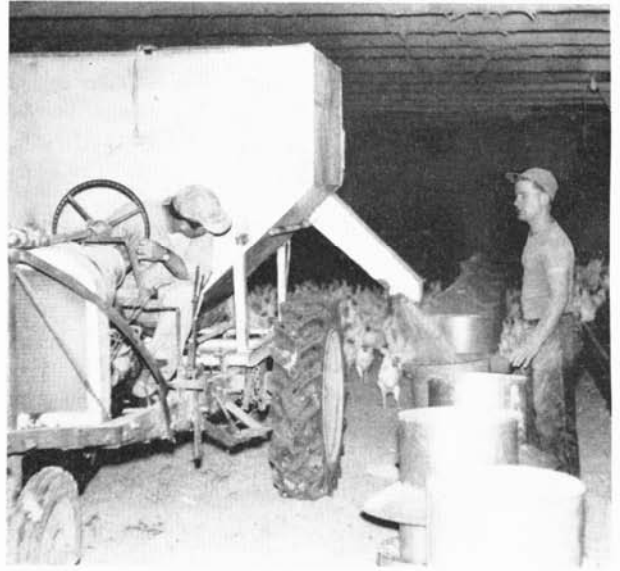
A self-unloading wagon brings feed from the processing center and augers it into self-feeders. The wagon can also be used for feeding other livestock.
