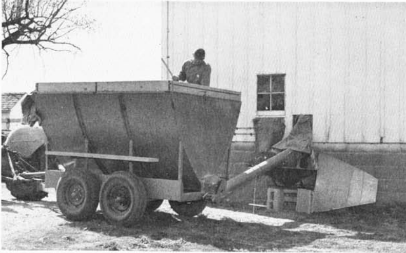
Ground feed in bulk is hauled from a mill in the neighborhood and augered to a storage bin on the fourth floor of this multiple-story house (left). The feed then flows by gravity into mechanical feeders on the lower floors (right).
