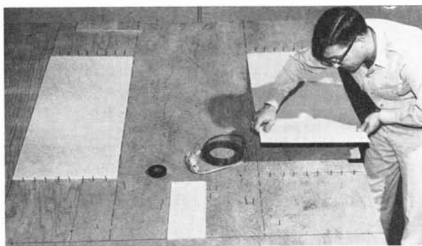
Placing cement asbestos panels on plywood jig.
