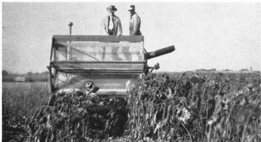
Here is a modified, small-grain combine doing a fair job of harvesting sunflowers. Plants are less than 5 feet tall, very uniform, and standing well. Reel blades are made solid with \frac{1}{2} -inch hardwood cloth. Sometimes other material, such as sheet metal or plywood, is used. (Fig. 2)
