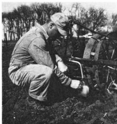
Using a quart measuring jar to determine the output of a nozzle in ounces per minute. (Fig. 11)
