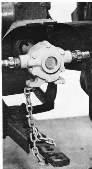
Using a short chain to prevent turning of the pump casing. (Fig. 12)
