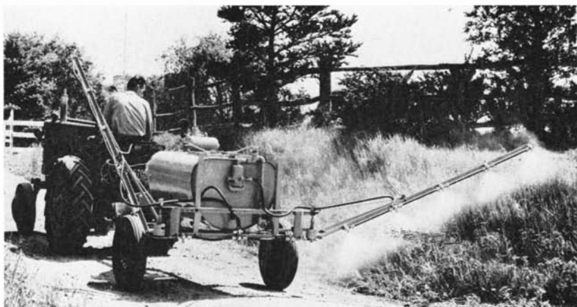
High nozzle pressure is causing excessive atomization of the spray and drifting that will damage ornamentals in the area. (Fig. 6)
