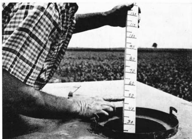
For tanks not marked at 5-gallon intervals, use a stick calibrated at 5-gallon intervals to find out how much solution is left in the tank. (Fig. 13)
