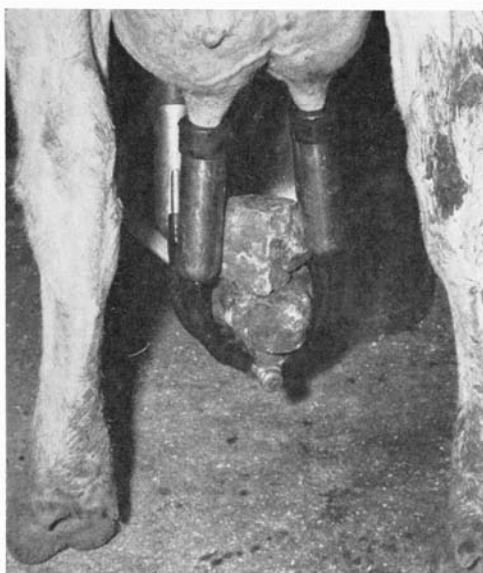
Because of inadequate vacuum reserve, rocks have been placed on this milker claw to add weight and thus help increase the rate of milking. (Fig. 3)
