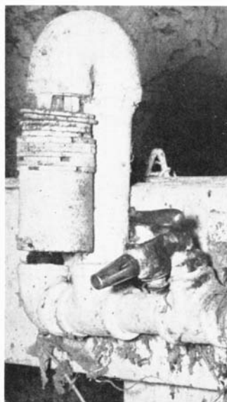
On more than half the farms, the vacuum control valve was at the end of the line. (Fig. 4)
