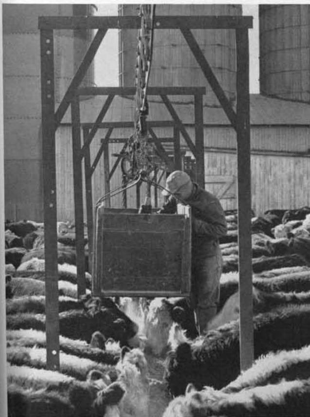
This farm-built carrier box has an adjustable opening in the bottom for feeding grain. The bottom is hinged at each end so that half or all of a load of silage can be dumped at once. The operator walks in the bunk to distribute feed.
