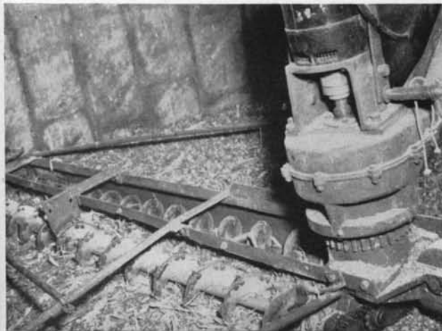
A mechanical surface unloader, using a screw conveyor to move the silage to the blower and conveyor pipe.
