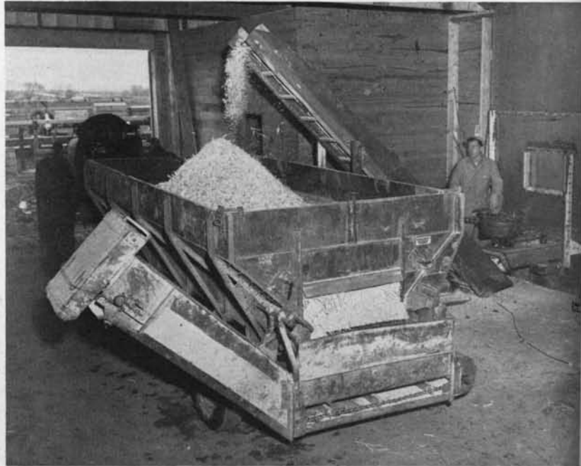
A self-unloading wagon is filled with silage by a mechanical silo unloader and elevator. Grain and supplement are added before moving to the feed bunks.
