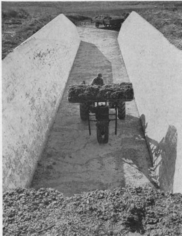
This farm-built power scoop (above and below) carries about 900 pounds of corn silage at a time. The scoop is loaded and dumped into the wagon rapidly and with little effort.
